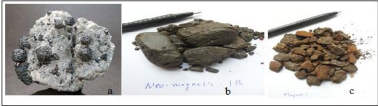
Figure 2.5 Tantalite ore (black) in pegmatite-spodumene mineral (a), concentrated Kenticha non-magnetic or tantalite (b) and magnetic or columbite (Mackay & Simandl, 2014; Nikishina et al., 2014)
