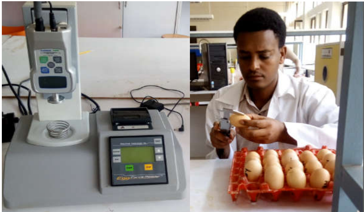
Picture 4: Equipment used to measure egg breaking strength and Measuring egg diameters and egg length (by micrometer screw gauge)
