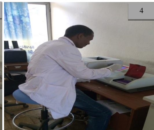
Set the wavelength, Control and labeling the whole samples accordingly
