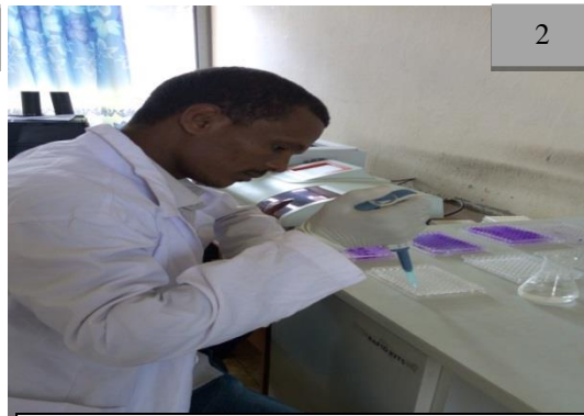
While dissolved CV transferred to new flat bottomed microtiter plate
