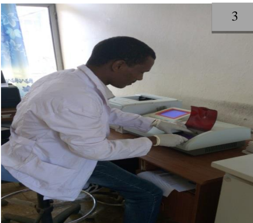
Insertion of microtiter plate into ELISA auto reader to measure absorbance
