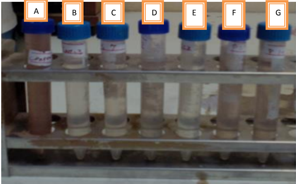
Figure 9 : Decolonization with different pH after agitated, centrifuged and filtered ready to read by spectrophotometry (A=control, B, C, D=pH (3, 7 and 10 using pumice and E, F and G=pH (3, 7 and 10 using scoria)
