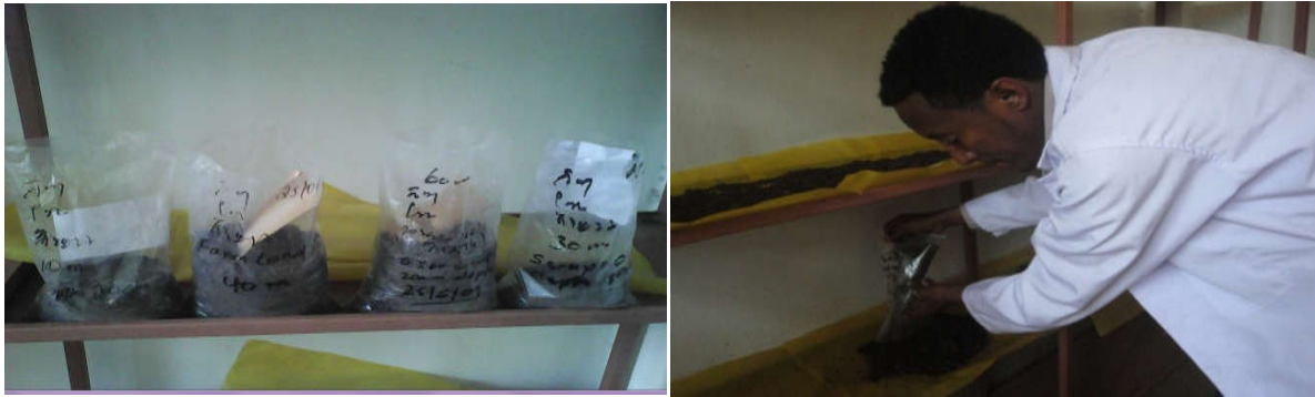
Figure 4: Soil samples in drying bed at soil laboratory.
