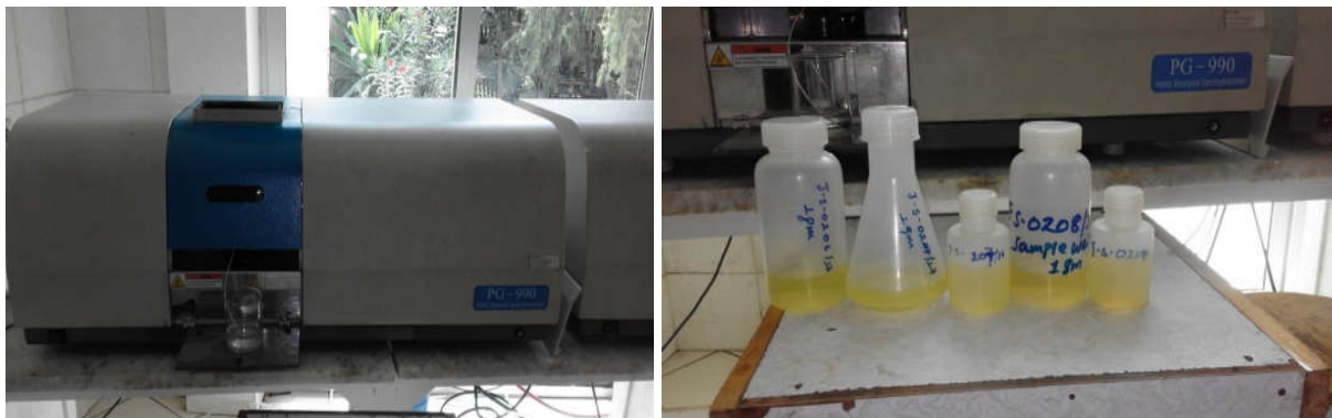
Figure 9: FAAS used for heavy metals measurement in JIJE analytical test service laboratory at Addis Ababa.
