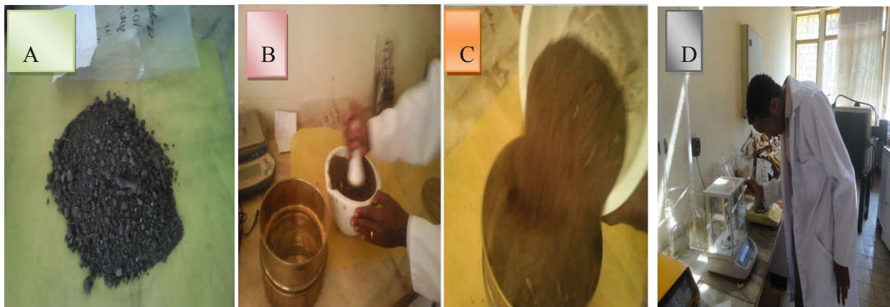
Figure 5: Soil samples treatment and preparation at laboratory.
