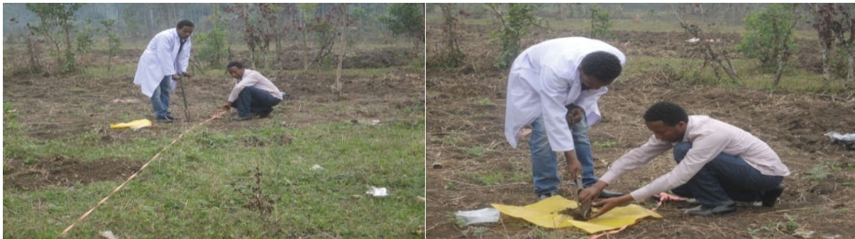
Figure 3: Soil sampling by hand augur at Teppi town solid waste dump site.
