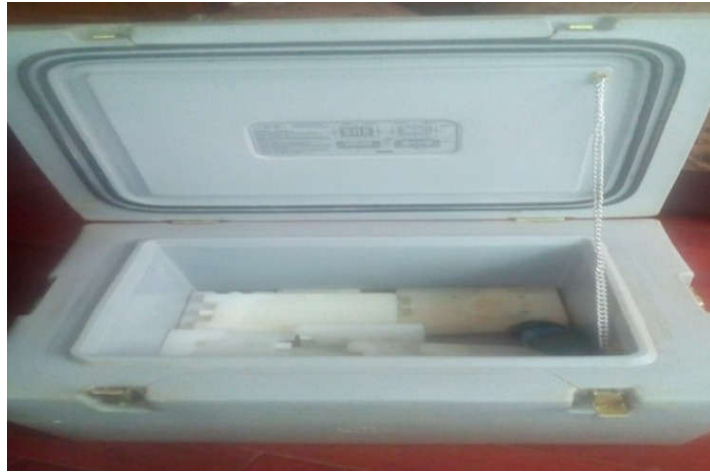
Figure 10: Model of Ice peg used for water and leachate samples preservation.
