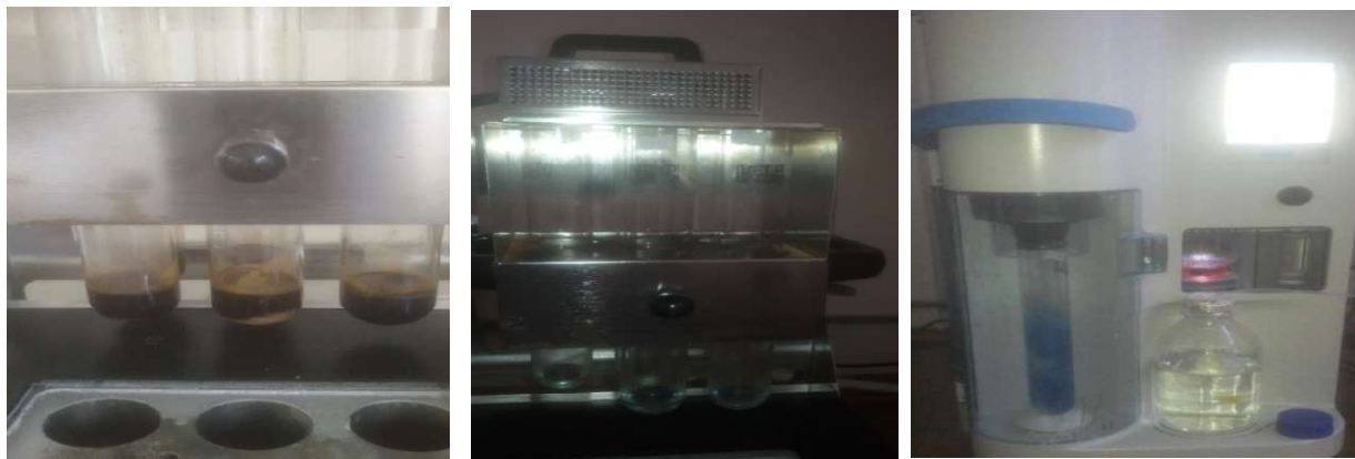
Sample with H 2 SO 4 ⇨ Sample after digestion ⇨ Sample distillation and Titration
