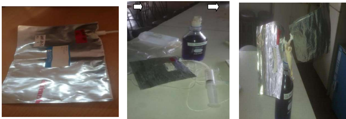
Sample gas containing plastic bag NaOH solution injecting of gas into solution
