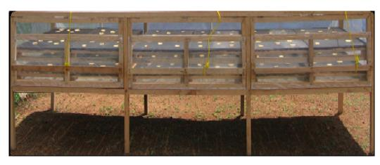
**Figure 1.** NRI-modified Kawanda solar cabinet dryer (front view) constructed at JUCAVM, Ethiopia. The dryer consisted of a main frame with eight supporting legs, incorporating the drying chamber covered with transparent polyethylene sheet. The drying chamber was 4.4 m long x 1.5 m deep x 0.8 m high overall and contains 12 trays to provide a total drying area of 10 m<sup>2</sup>.
