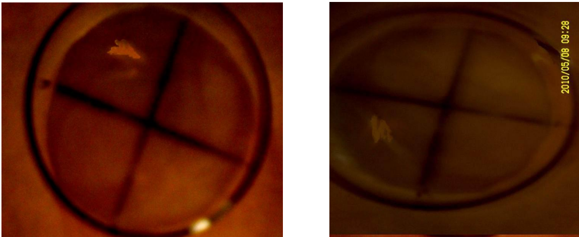
Figure 5.1 Qualitative screening result of Sphingomonas strain LBG-5 (left) and fungal strain LBG-10 (right). The clearing of the color of the plastic disk indicates degradation of the material by microbial action.
