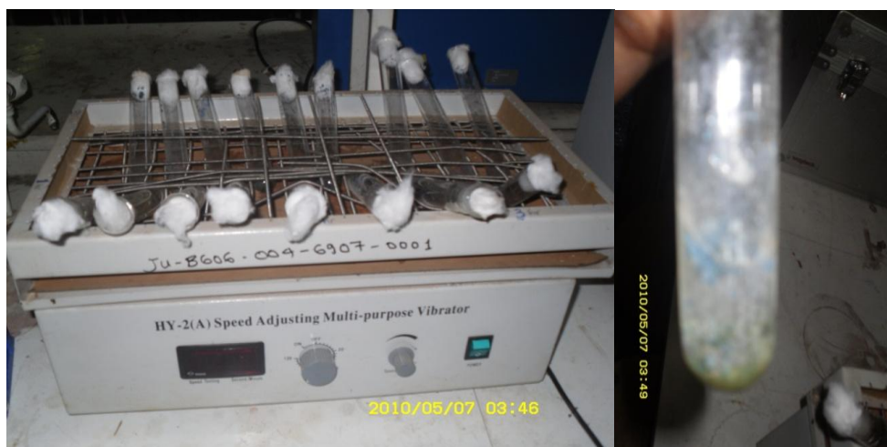
Figure 4.1 Isolation of plastic-degrading microorganisms using polyethylene. Left, incubation with shaking of the enrichment medium; Right, close-up of medium showing PE plastic as carbon source.
