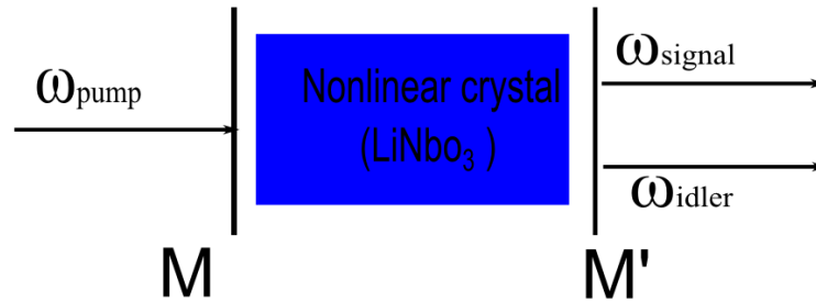
Figure 2.4: Diagram of optical parametric oscillation
