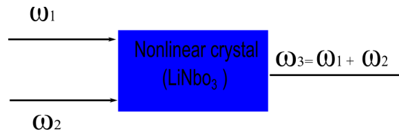
Figure 2.2: Geometry of interaction for sum frequency generation
