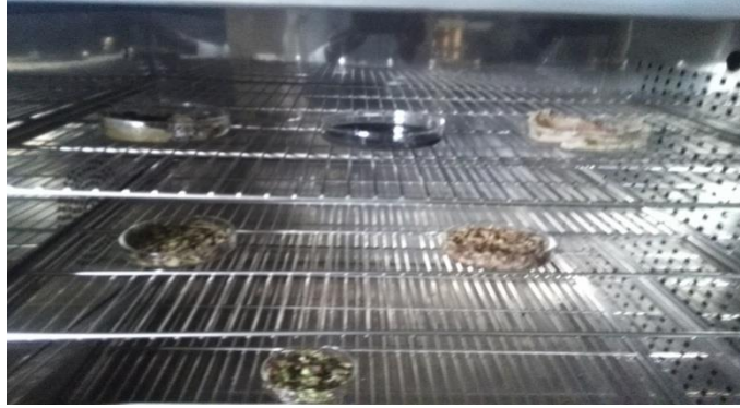
Figure 3: Drying samples using hot air oven
