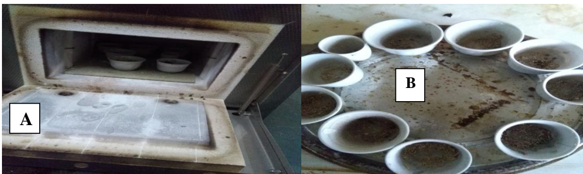
Figure 4: A. Drying samples using furnace, B. Remaining mass after ignition
