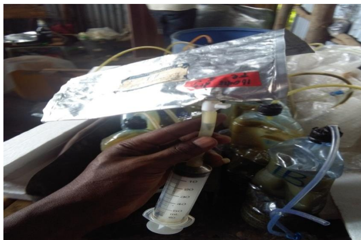
Figure 8: Collecting biogas for methane determination
