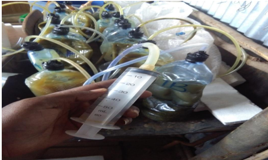
Figure 1: Sucking air by syringe to maintain anaerobic digestion
