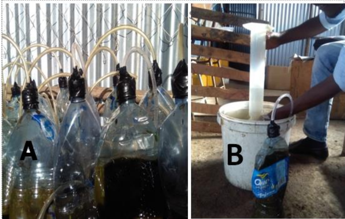
Figure 2: A: Triplicate arrangement of digester, B: Determination of biogas by water displacement method
