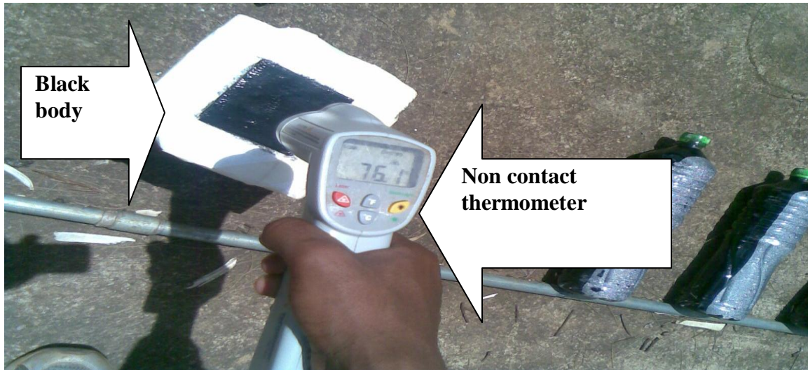
Figure 8. Solar irradiance measurement by non contact thermometer and black body, June, 2011, Jimma, Ethiopia.
