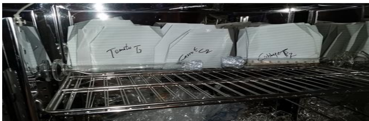
Figure 3: sample drying in oven for metal analysis
