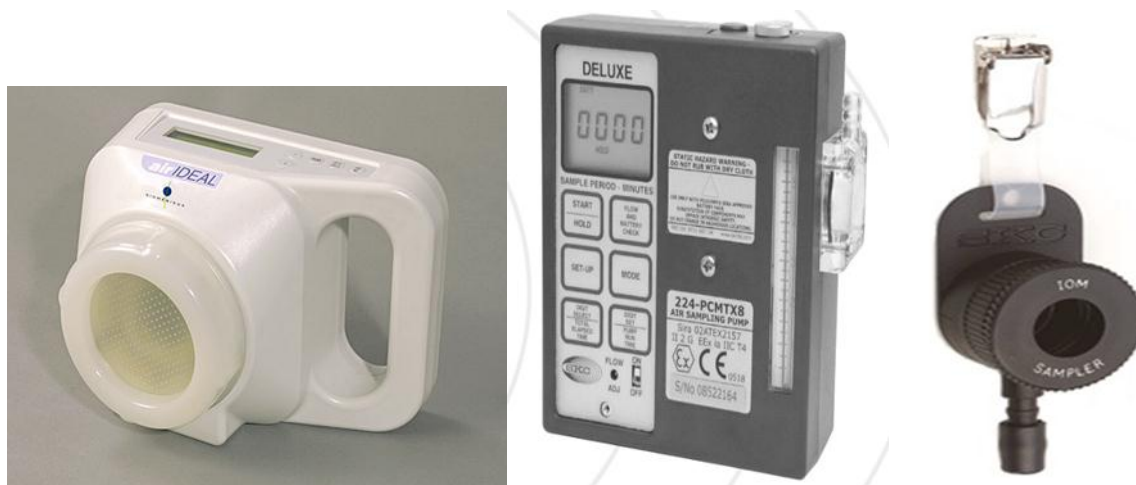
Figure 3. In the left is Air IDEAL sampler and in the right is Universal Air Sampling Pump
