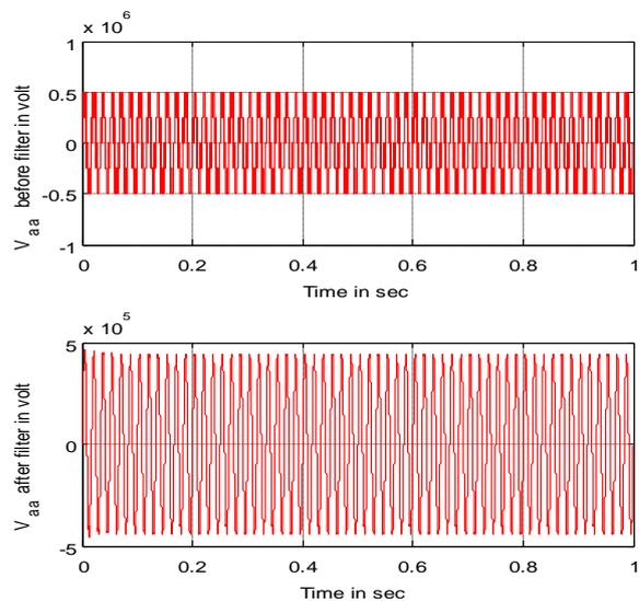
Fig.5. Voltages across inverter terminal under normal condition
