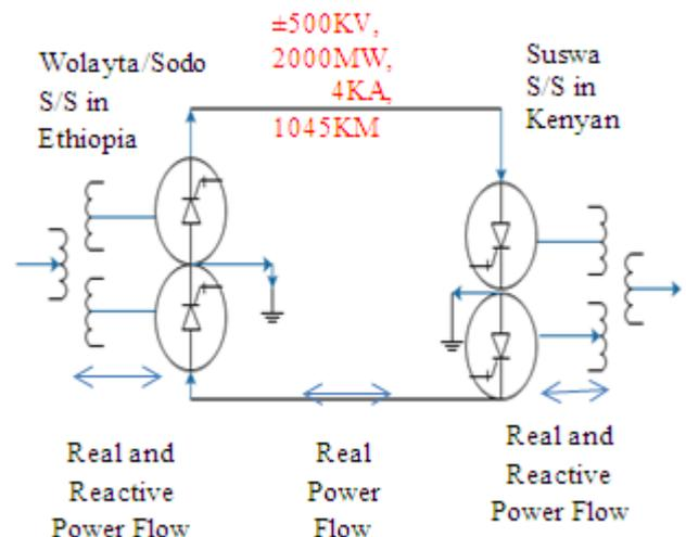
Fig.1. HVDC system based on VSC technology built with GTOs
