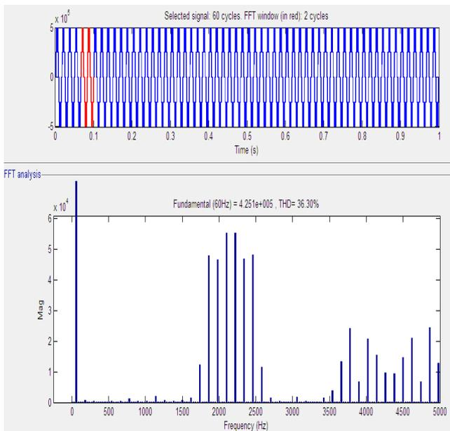
Fig.7. Harmonics spectrum of inverter voltage without filter
