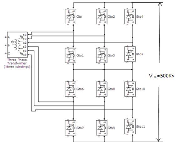
Fig.2. Twelve pulse valve group configuration
