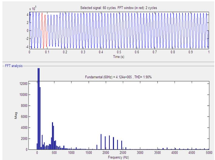
Fig.8. Harmonics spectrum of inverter voltage with filter
