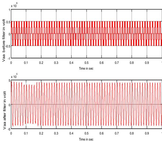
Fig.6. Voltages across the inverter terminal under fault condition
