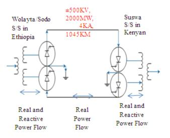
Fig.1. HVDC system based on VSC technology built with GTOs
