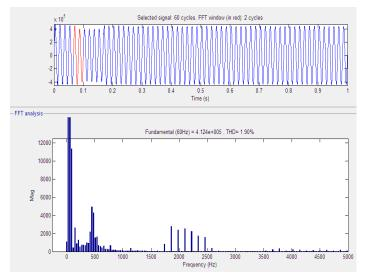
Fig.8. Harmonics spectrum of inverter voltage with filter
