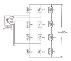
Fig.2. Twelve pulse valve group configuration
