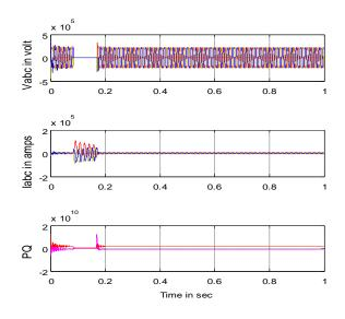
Fig.4. Voltages, Current, and Power under fault condition
