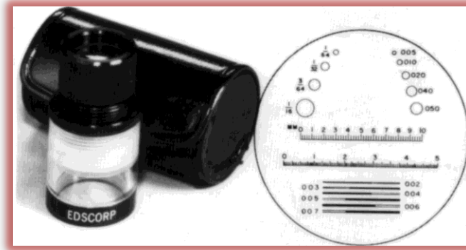
Figure 19 Comparator for measuring cracks widths (courtesy of Edmund Scientific Co.)
