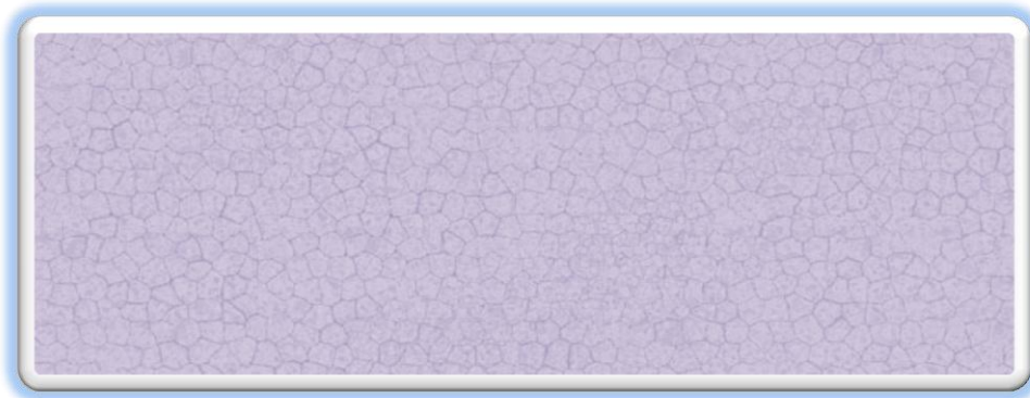
Figure 12 Crazeing pattern [Image Credit: Victoria Interval]
