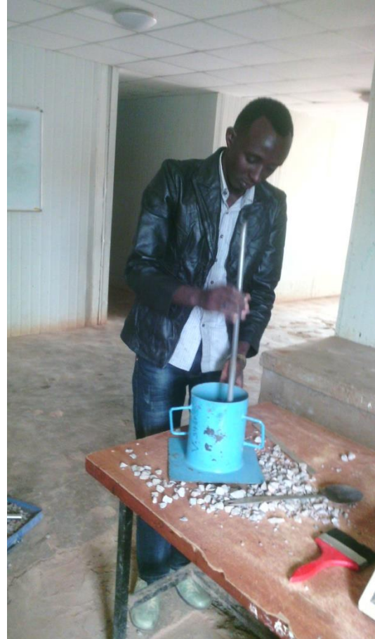
8. Dry rodded and loose unit weight determination
