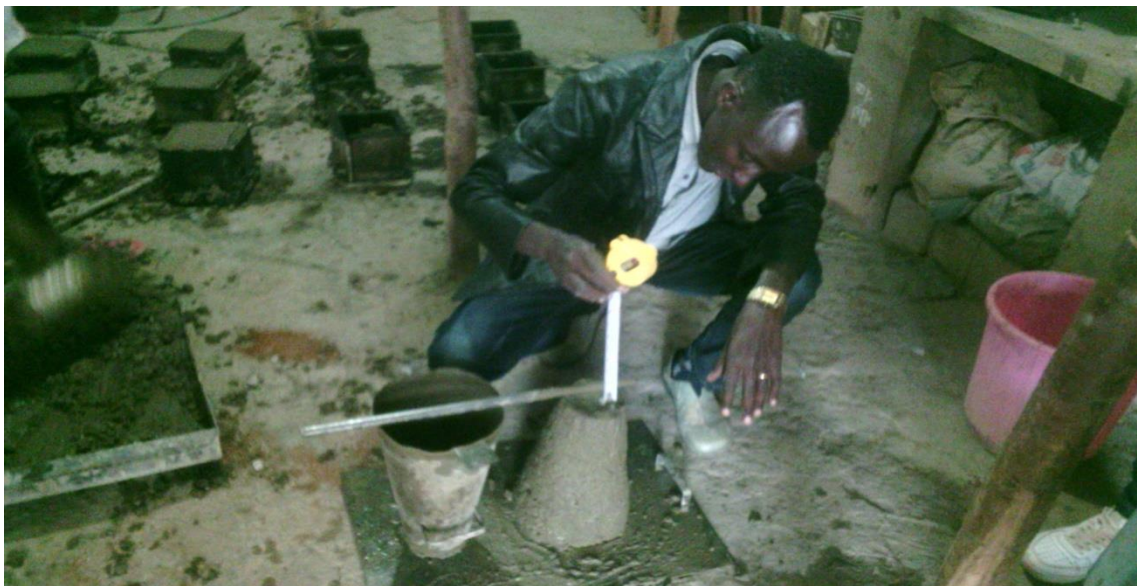
Fig 3.3. Measure of Concrete workability using slump cone
