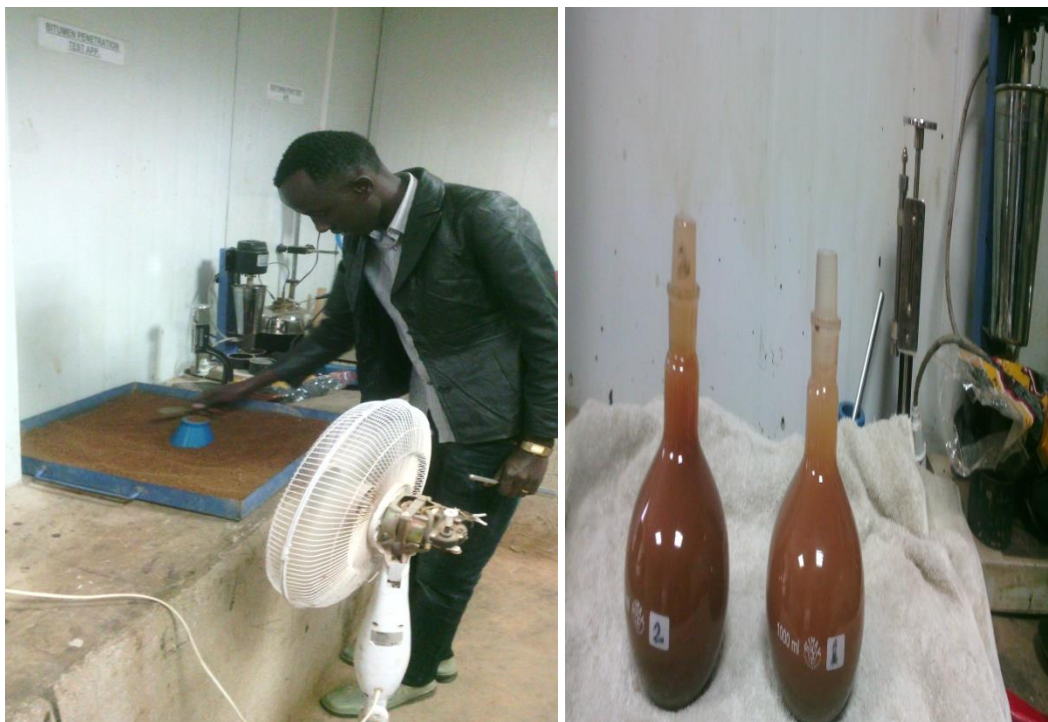
Fig 4.4. Determination of specific gravity of Moyale river sand
