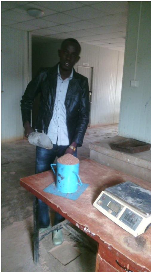
8. Dry rodded and loose unit weight determination
