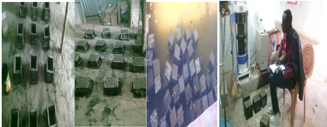
Fig.4.9. Steps in cube tests from left to right: greasing of mold, casting, curing and crushing
