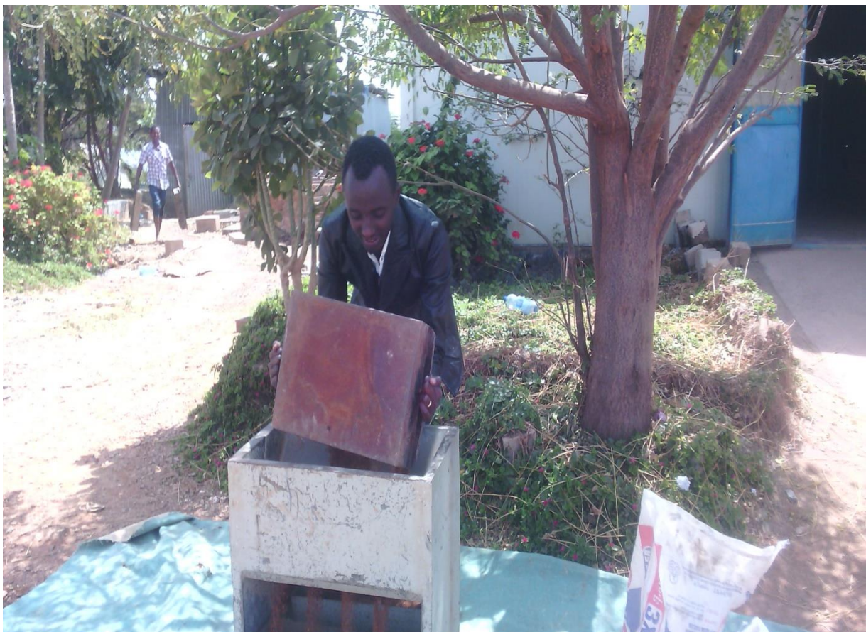
7. Sample quartering using riffle box prior to any experiments
