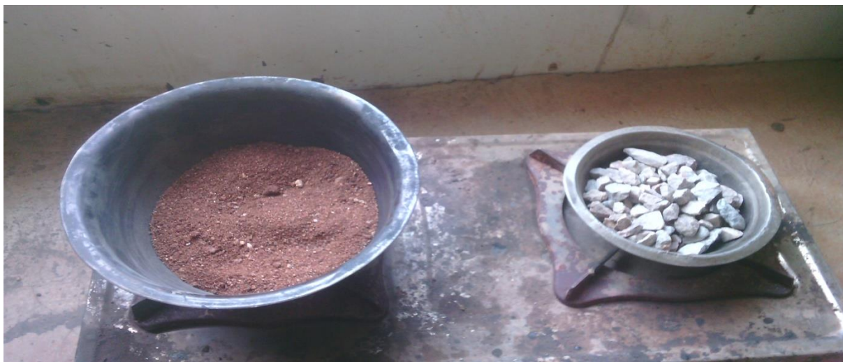
Fig 4.5. Natural moisture contents determination
