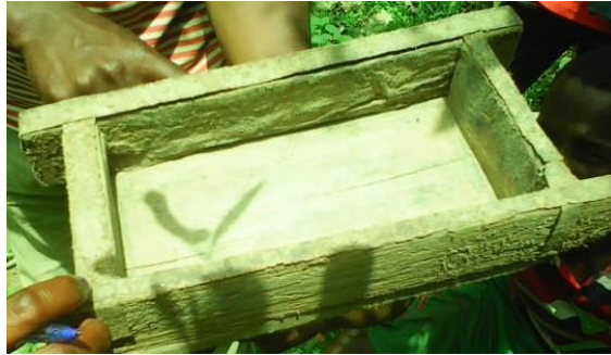
Fig.3.5.3.1. “Stampa” a locale brick production mold in Jimma town
