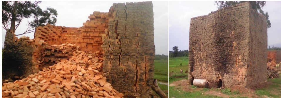
Fig.3.5.1. local firing process of bricks
