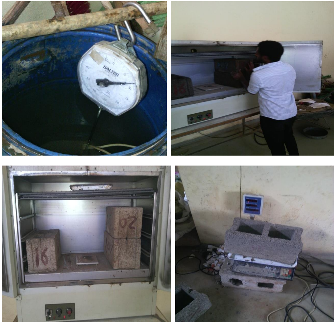
Figure 4.3.4 density, moisture content & absorption test
