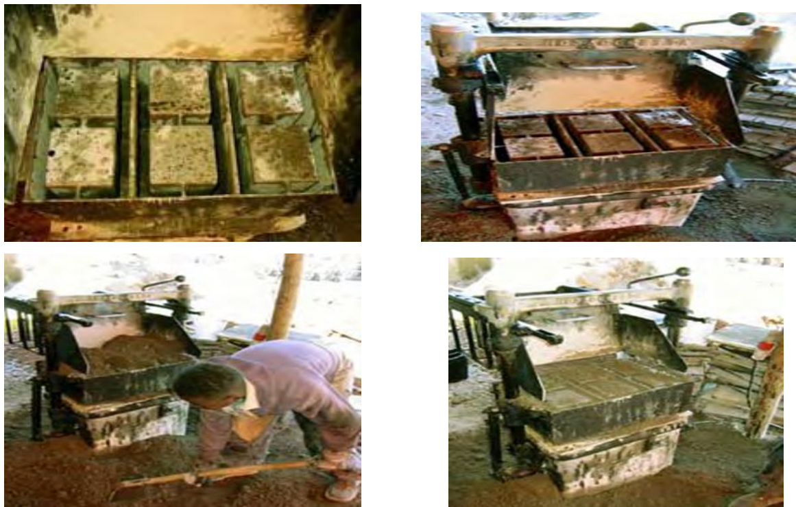
Figure 2.5.1 Casting procedure and casting machine
