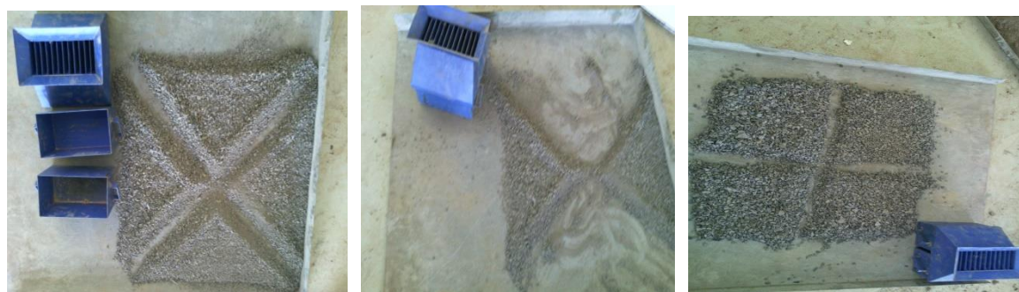
Figure 3.3.4 quartering and sample splitter for crushed aggregate
