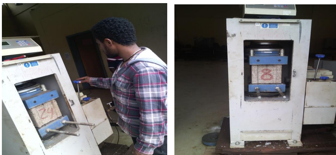
Figure 4.3.1 laboratory test of HCB
