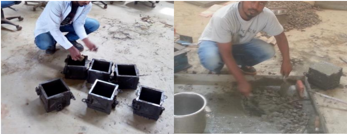
Figure 3.2: A and B shown scrubbing the mold with oil and mixing the ingredients respectively
