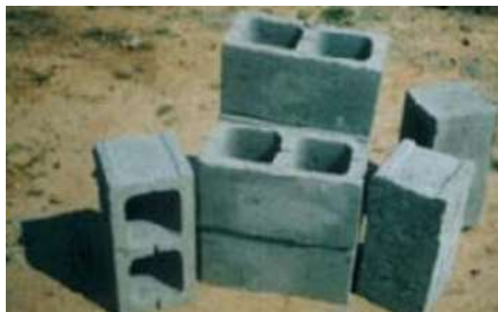
Figure 1: Hollow concrete blocks (source: - SRCCD, 2008)
