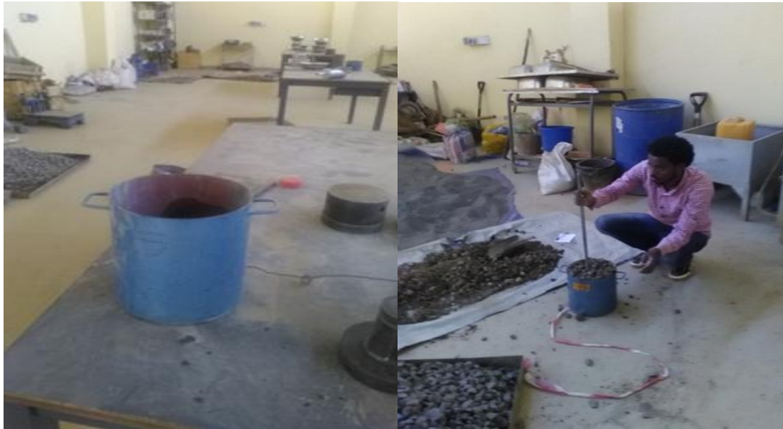
Figure 3.9 Bulk Density of coarse Aggregate Test both river gravel and crushed coarse aggregate.
