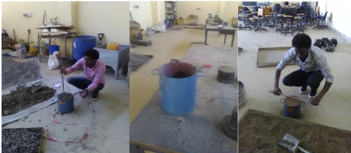
Figure 7: Dry-Rodded Unit Weight test of fine and coarse aggregate
