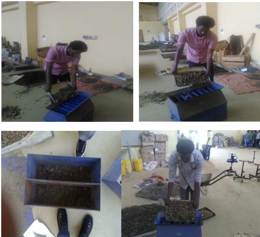
Figure 4: splitter or reducing aggregate field sample to test size of river gravel and crushed coarse aggregate
