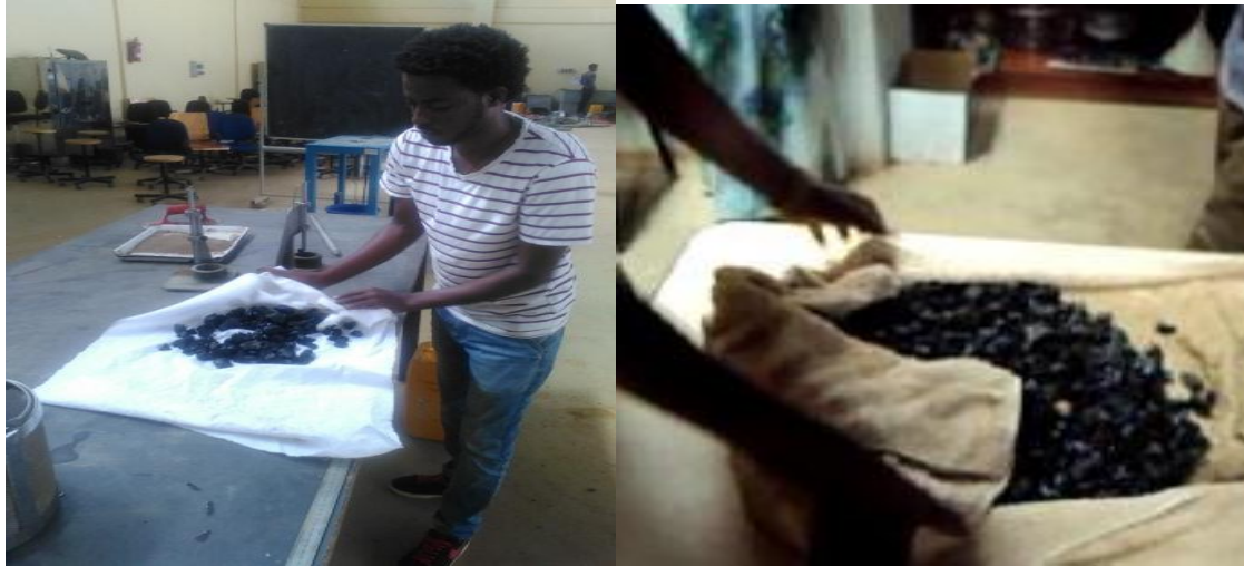
Figure 6: Specific Gravity (SSD) and Water Absorption test for river and crushed coarse aggregate
