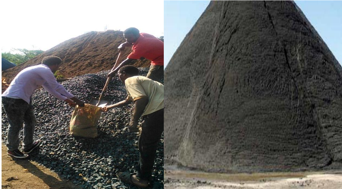
Figure 1: Crushed coarse and fine aggregate field sample from varnero aggregate crusher site
