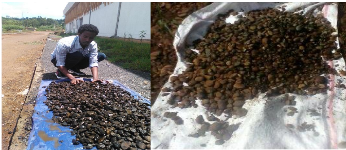
Fig 2 Washing river gravel aggregate
