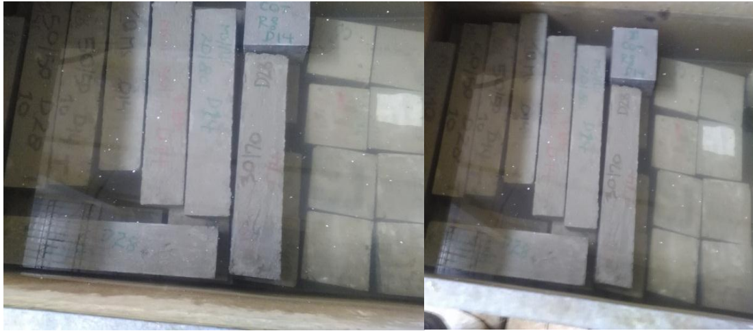
Fig 15 curing of cubes and beams at different age
