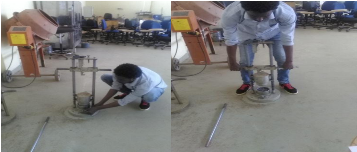
Figure 9: Aggregate Impact Value test for natural gravel and crushed coarse aggregate
