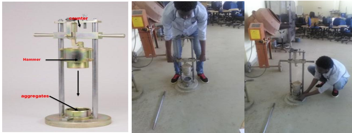
Figure 3.10 Aggregate Impact Value test
