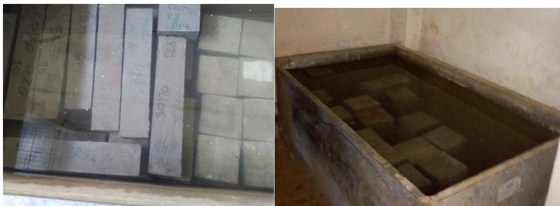
Figure3.13 Curing cube and flexural beam
