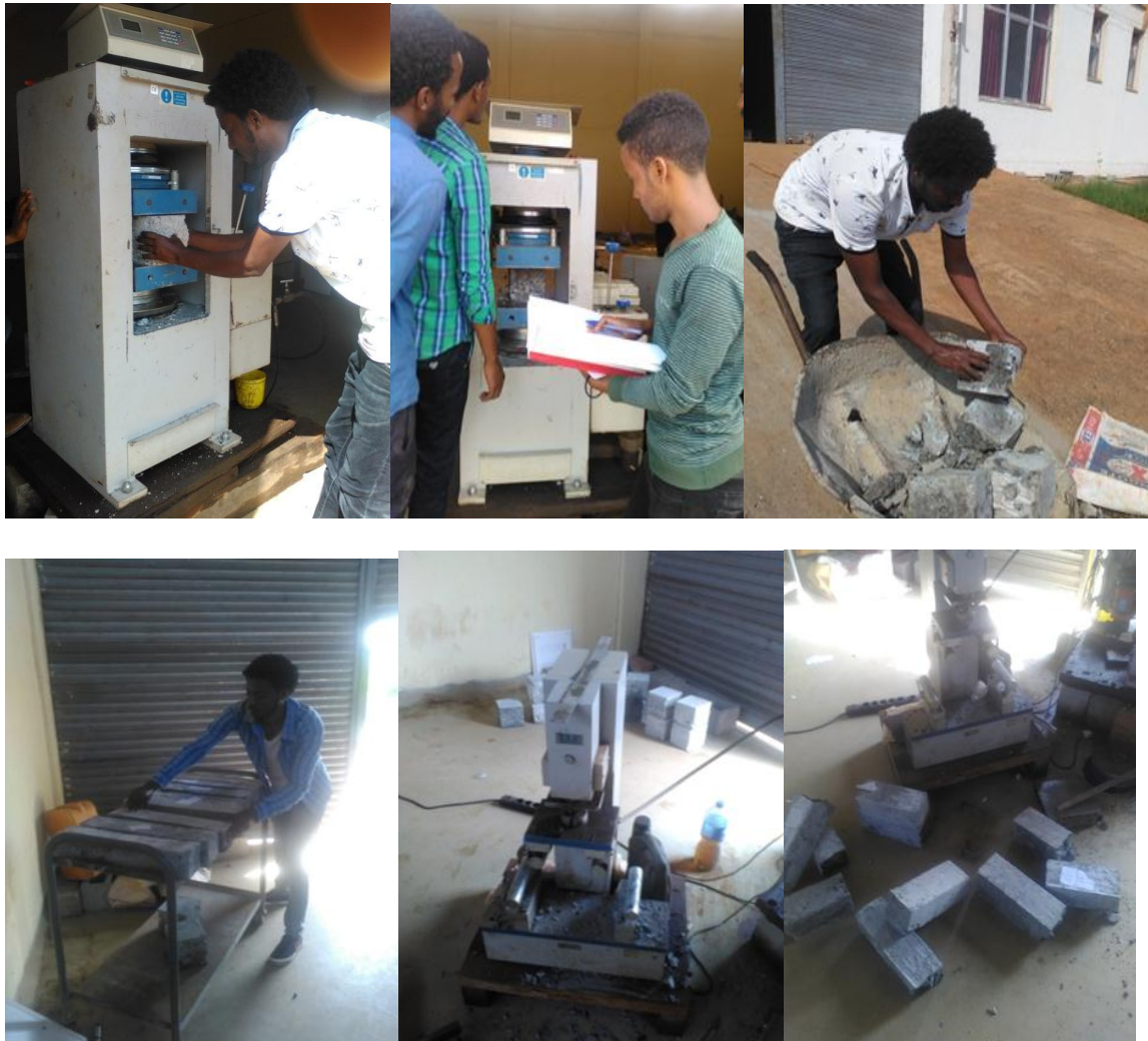
Fig 16 compressive and flexural strength test
