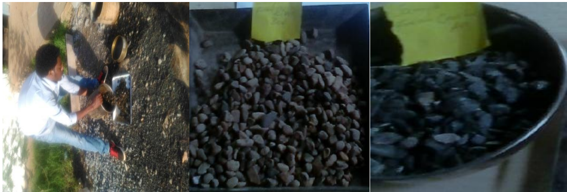
Figure 5: Sieve Analysis; Gradation coarse aggregate
