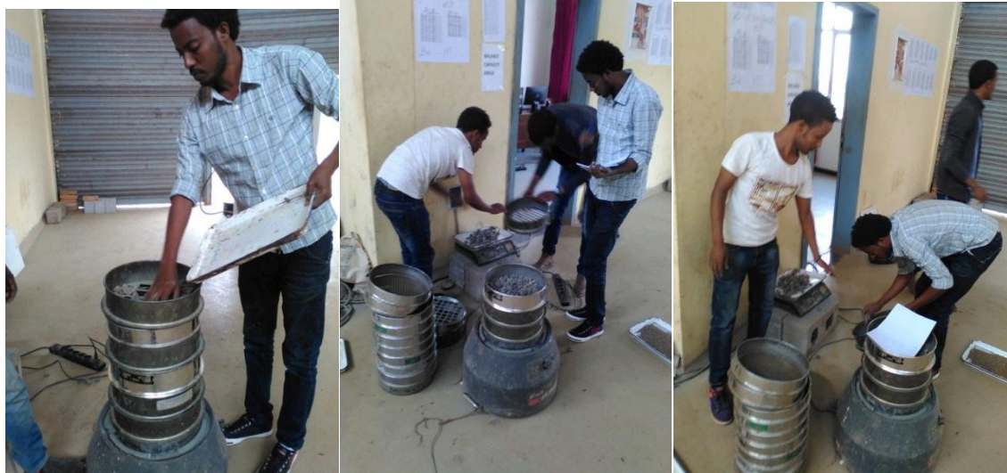
Figure 5: Sieve Analysis; Gradation coarse aggregate
