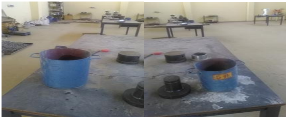
Figure2.5 The Cylindrical Metal Measures bulk density for the Fine and Coarse Aggregates [28]
