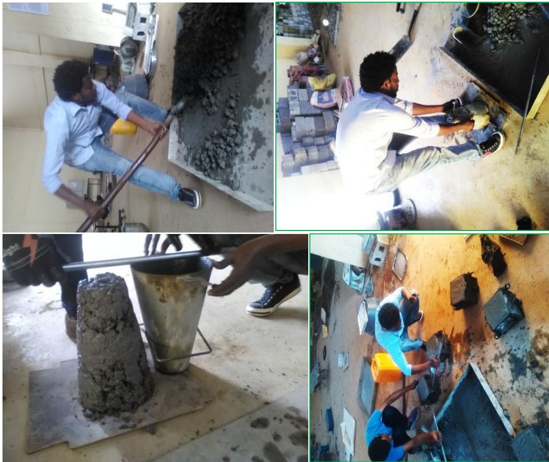
Fig 14 casting cubes and slump test
