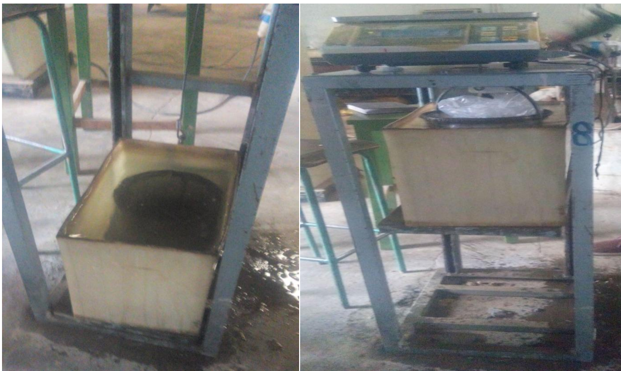
Figure 3.3: Specific gravity of coarse aggregate, process of Immerse the basket with the sample
