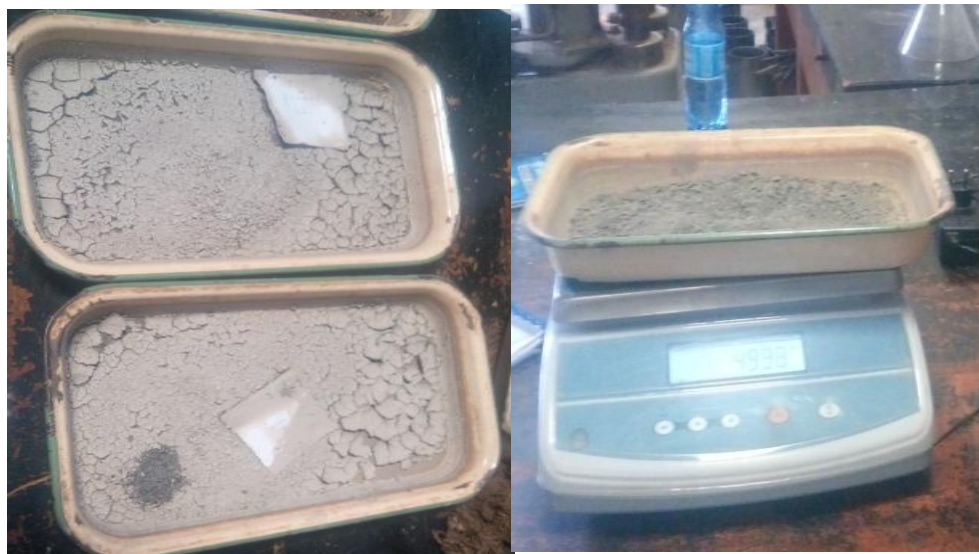
a) Oven dry sample b) Weight of oven dry sample
