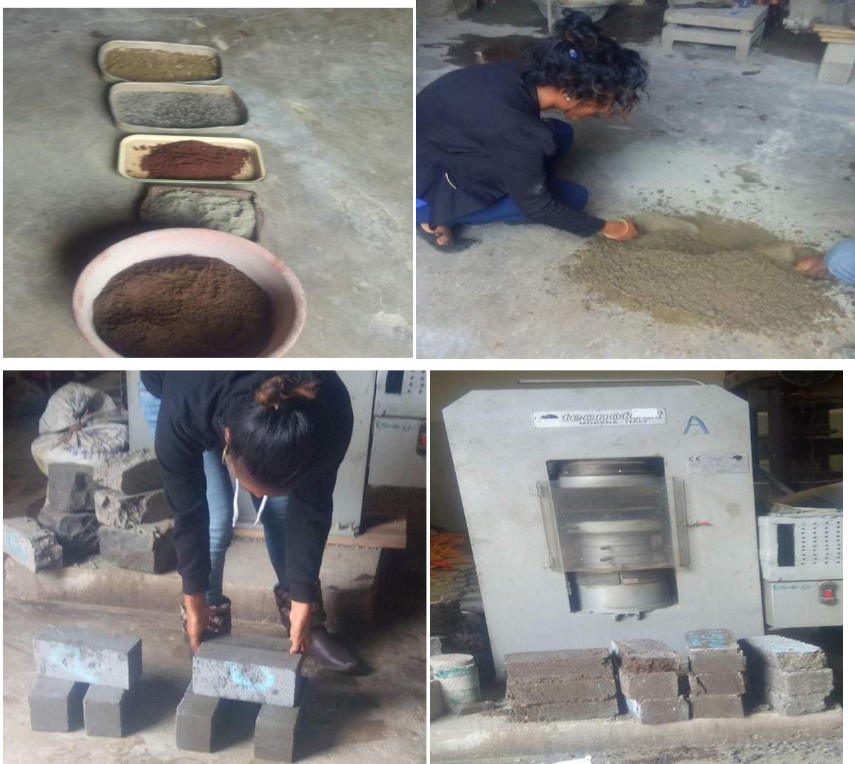
Figure 3.10: measuring and mixing of sample for first trial and compressive strength of sample
