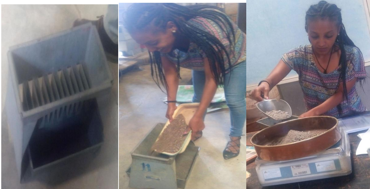
Figure 3.1; Quartering method and measuring samples
