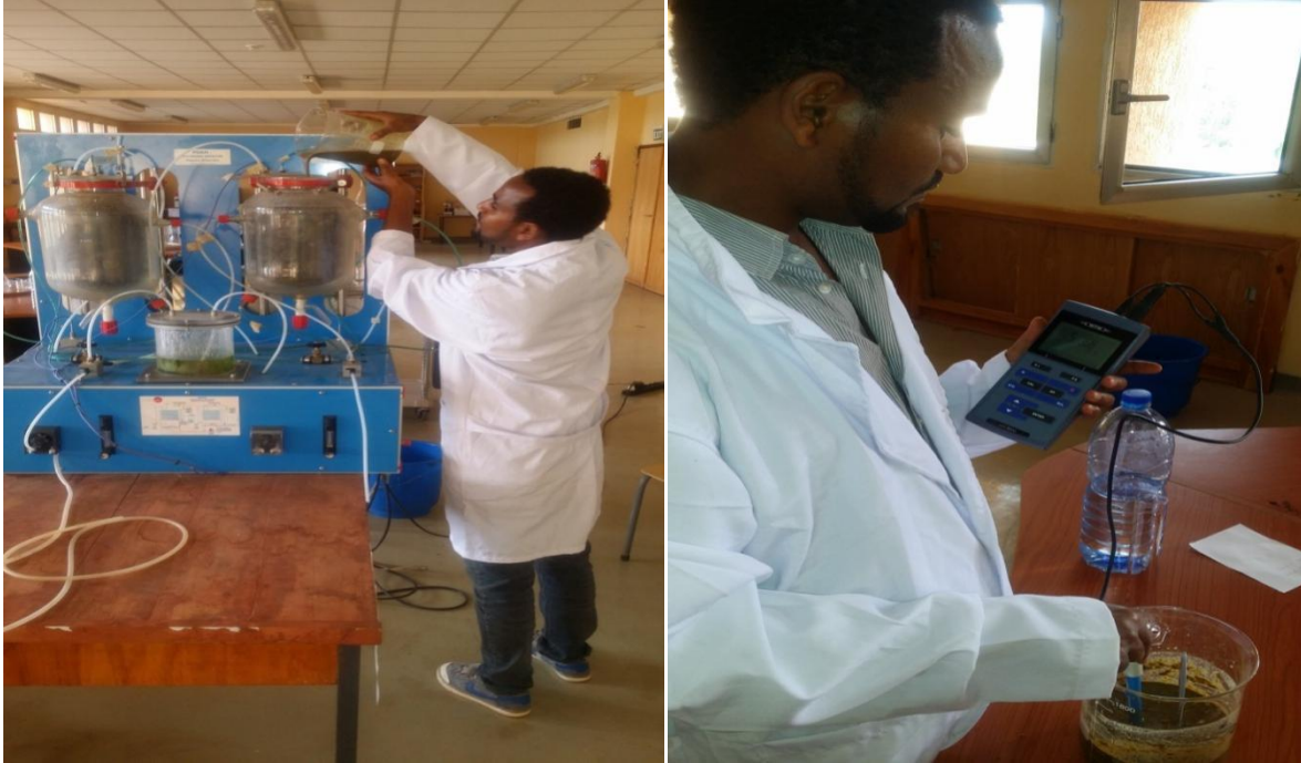
Figure 3: Stock solution pH adjustment and feed to the digester
