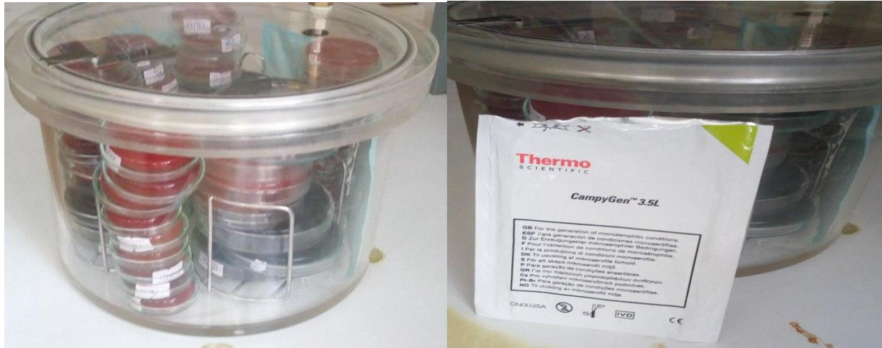
Figure 5: Incubation of an inoculated medium at microaerobic environment using anaerobic jar and 3.5L sachet
