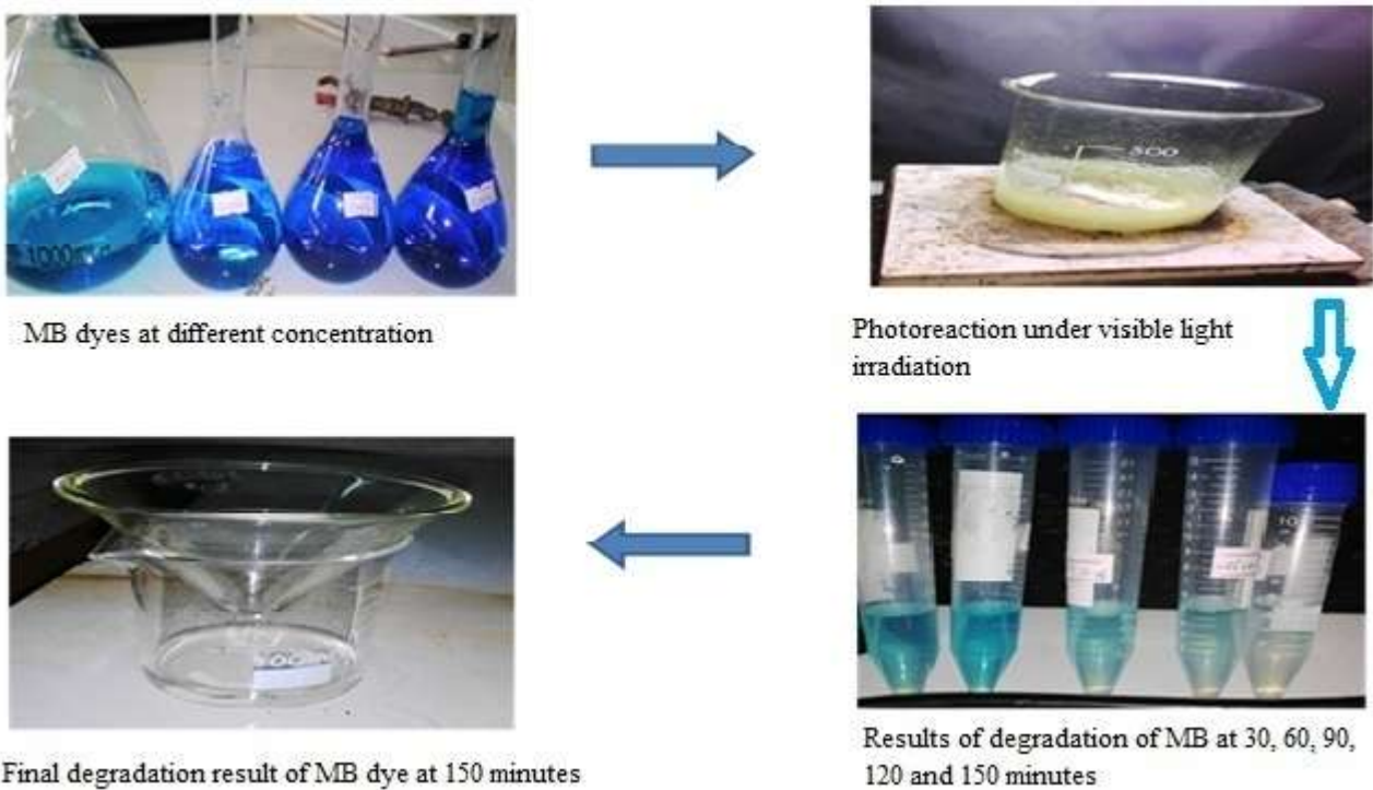
Figure 15. Degradation of MB dye using \text{ZnO-Ag}_3\text{PO}_4\text{-Fe}_2\text{O}_3 (80:10:10) nano photo-catalyst.
