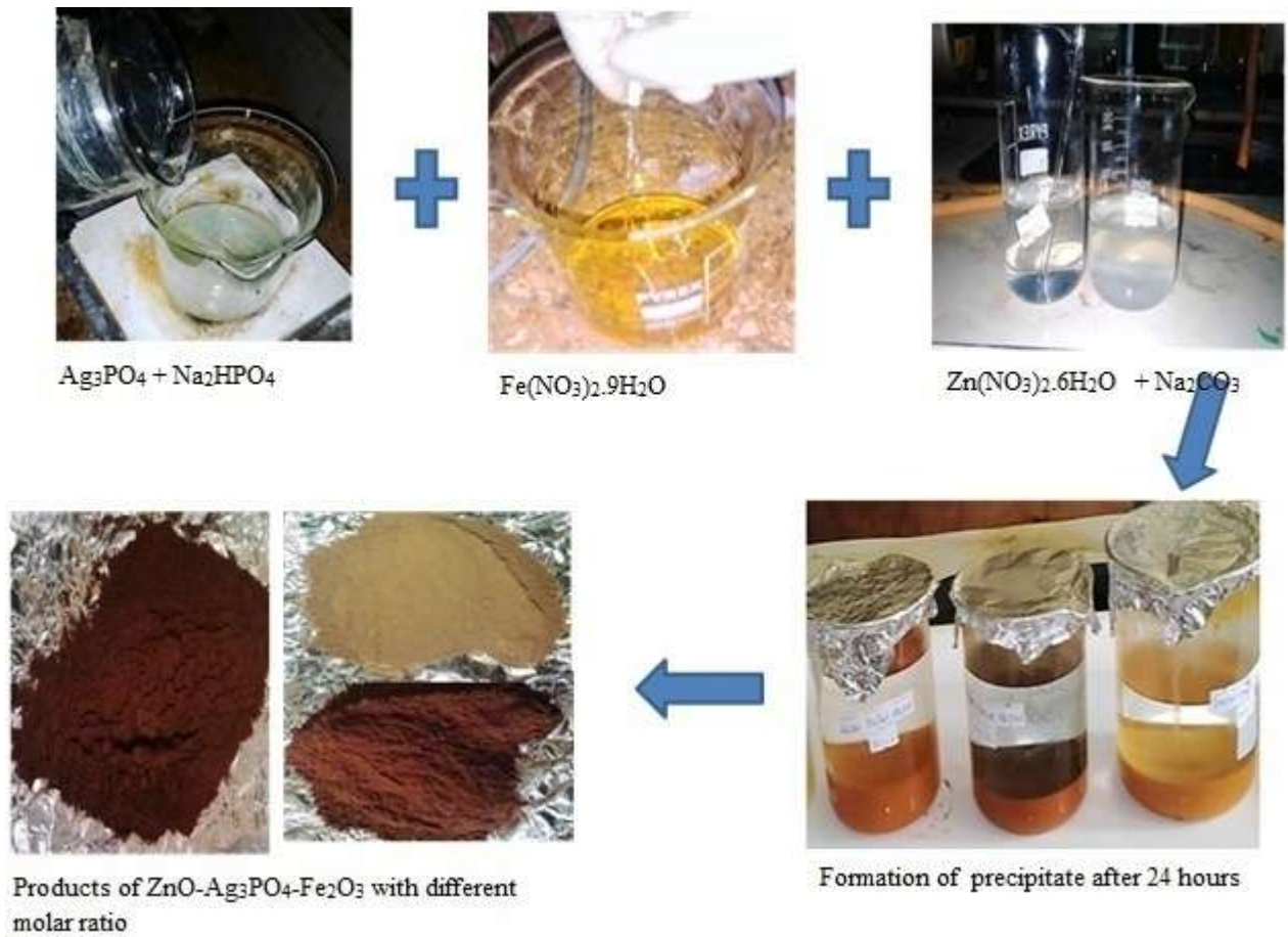
Figure 14. Preparation of \text{ZnO-Ag}_3\text{PO}_4\text{-Fe}_2\text{O}_3 ternary nanocomposite at different molar composition
