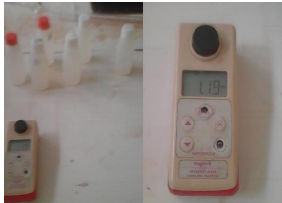
Measuring turbidity of water sample
