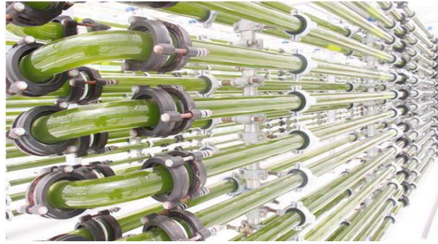
Figure 2.6: Close photo bioreactor system of microalgae cultivation (adapted from: (Chisti, 2007).
