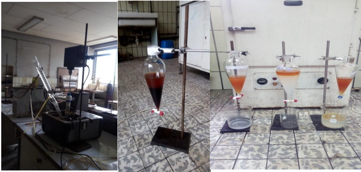
a) Stirred device b) biodiesel with glycerol oil c) washing of biodiesel
