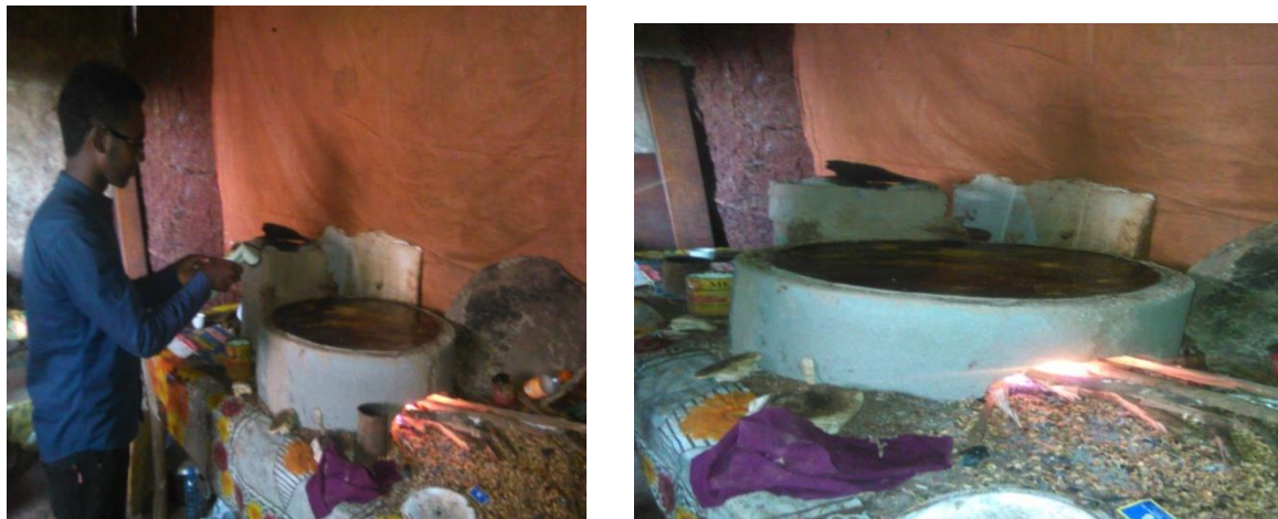
Figure 3.2 By using infrared thermometer the initial and final temperature of the stove were recorded
