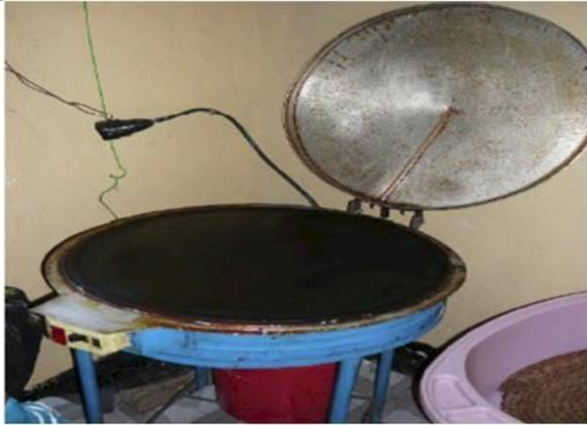
Figure 2.7 Electrical Injera baking mitad assembly
