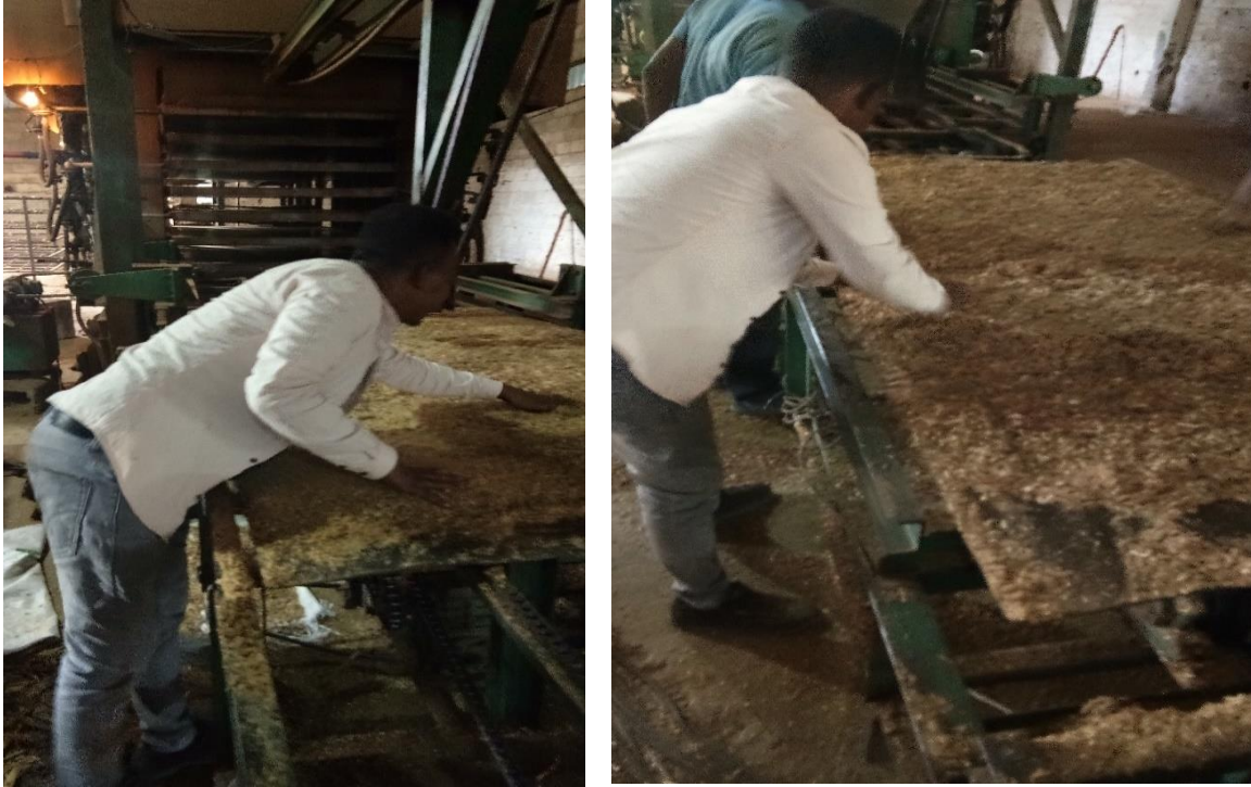
Figure 3. 3 Hand layup (mixing)
