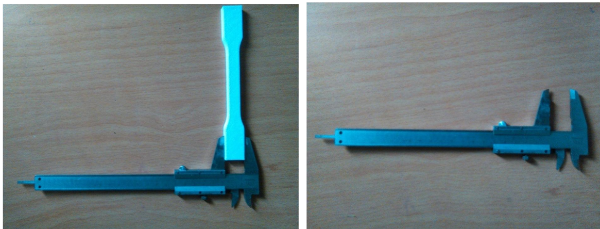
Figure 3.9 Test sample for dimensional analysis
