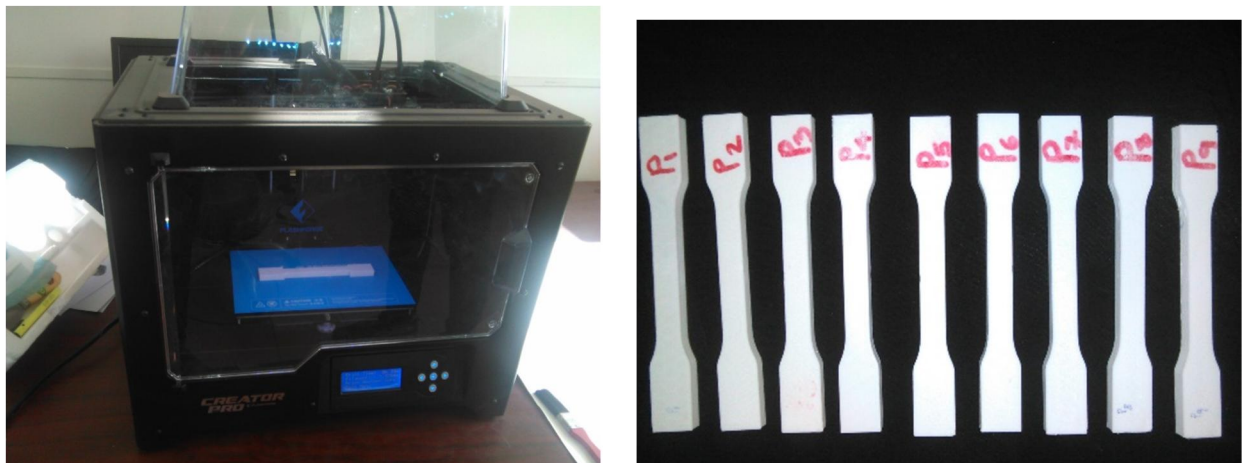
Figure 3.7 Parts fabricated by FDM machine
