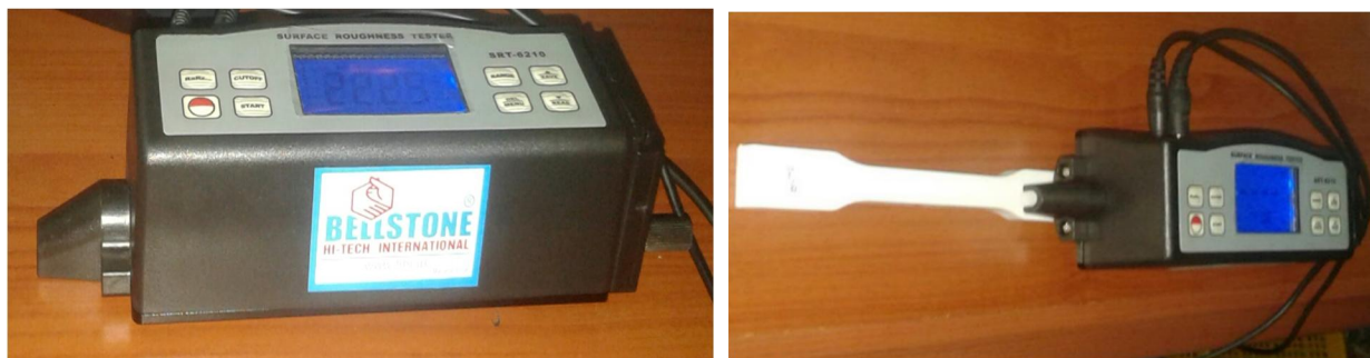
Figure 3.10 Measurements by BELLSTONE to the parts produced by flash forge FDM
