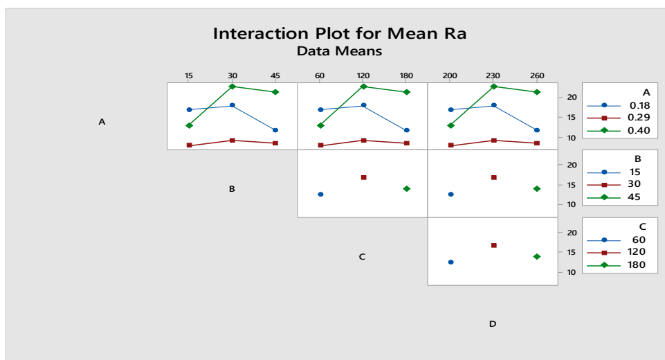
Figure 5.3 Interaction plot for Ra means with all process parameters
