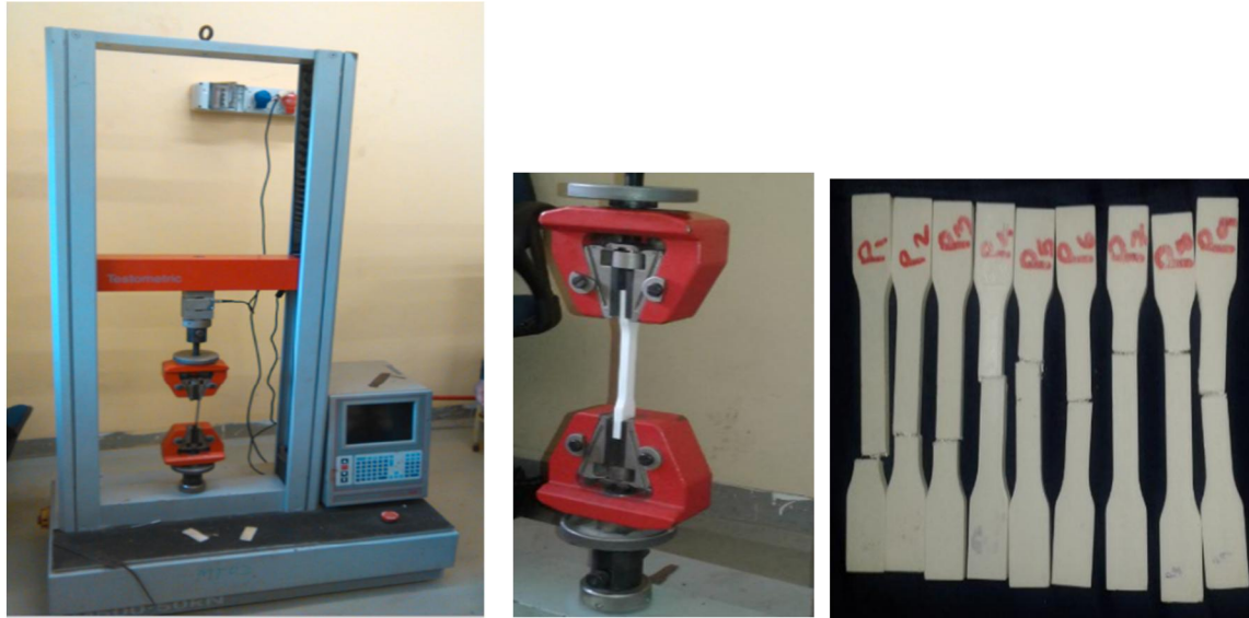
Figure 3.11 Testometric Machine and tested specimen
