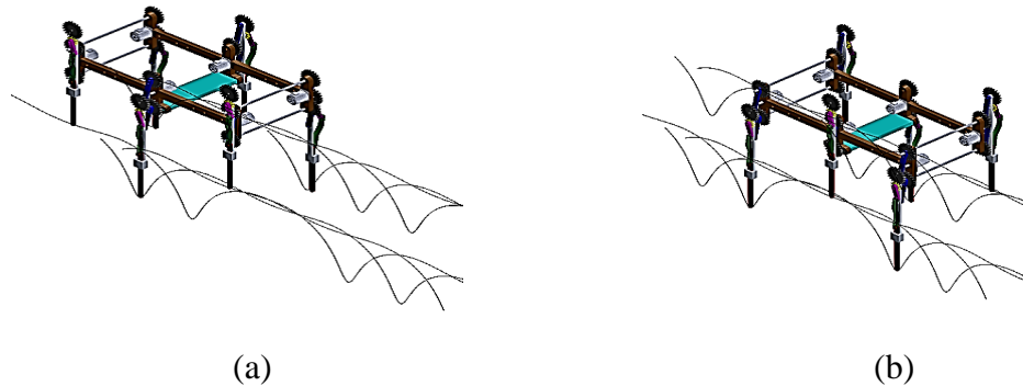
Fig. 31. Motion path for CAD model: (a) First three legs (b) Second three legs
