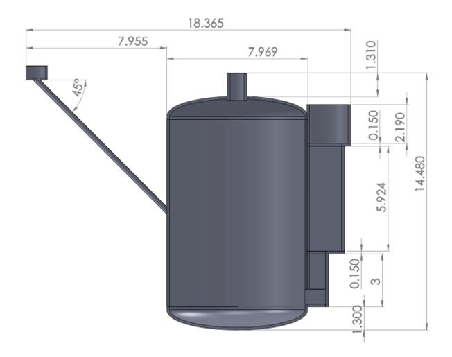
**Fig.6 Overall Dimension of Digester**
