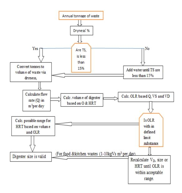
Fig.1 Process flow chart used to determine the required digester size [35].
