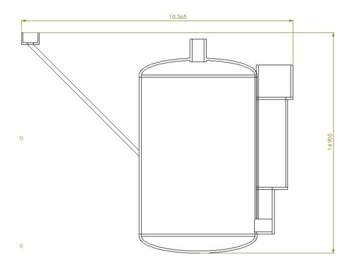
Fig.4 Dimension of Digester (L X W)
