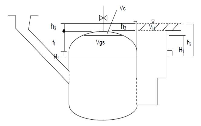
Fig. 3.16 Volume of hydraulic chamber, gas collecting chamber and gas storage chamber
