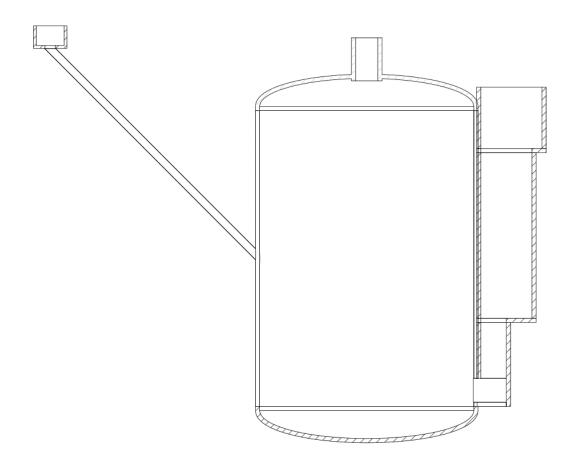
Fig.2 Cross section of Digester
