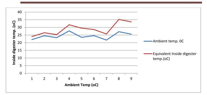
Fig 4.3 Graph of measurements of inside digester temperature and ambient temperature at different days (at Experiment one)
