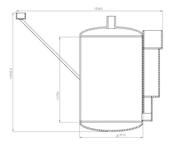
Fig.7 Some Cross sectional dimension of digester
