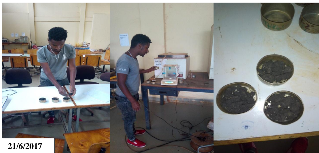
Figure 3.8: Determination of Natural Moisture content
