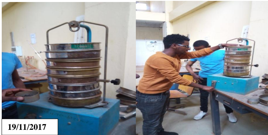
Figure 3.11: Sieve analysis (photo captured by Dakebi G.)
