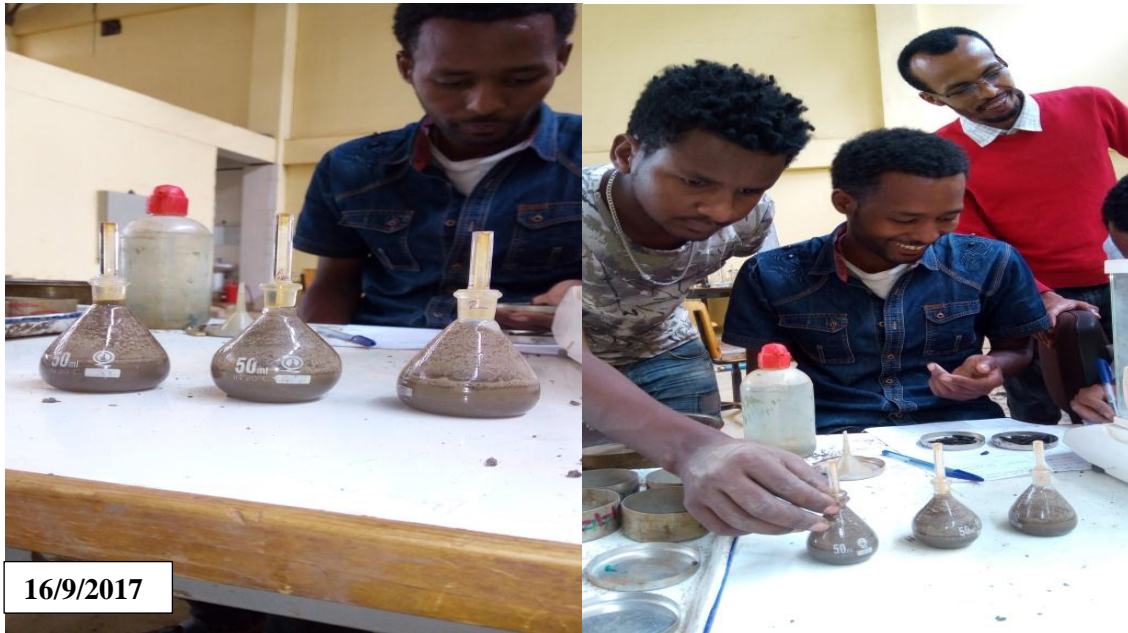
Figure 3.13: Determinations of specific Gravity (photo captured by Bona A.)
