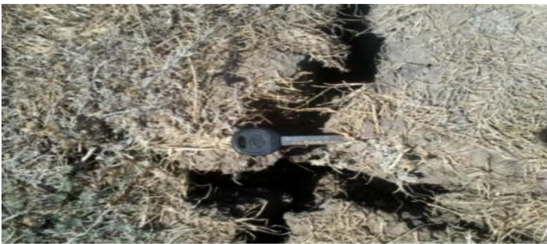
Figure 2.8: Polygonal cracks on the ground surface during dry season of expansive soil (Tagel, M., 2016)
