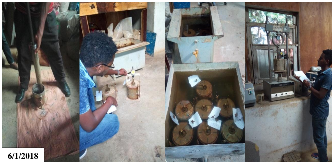
Figure 3.10: CBR test Procedure (photo captured by Nisar M.)
