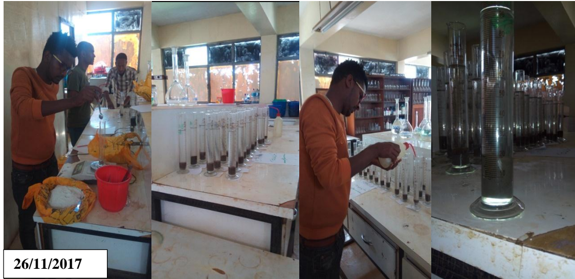
Figure 3.14: Free swell test Procedure (photo captured by Dekebi G.)
