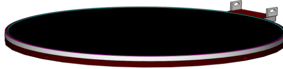
Figure 21: Conventional electric mitad with edge barrier
