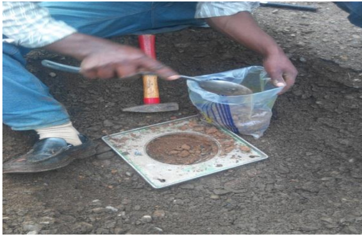
Figure 3.4 field density tests (photo 9, 7, 2016)
