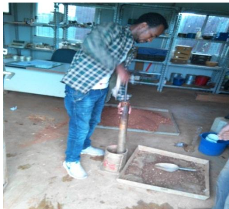
Figure 3.6 Procter test (photo 17, 7, 2016)
