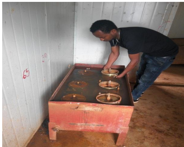
Figure 3.7 soaking of sample for four days (photo 18, 7, 2016)
