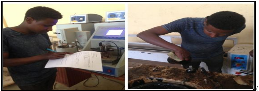
Figure 3.5 Softening point of bitumen and specific gravity test of bitumen
