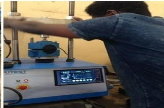
Figure 3.13 Prepare specimens for Test and Digital Marshall Flow stability test respectively
