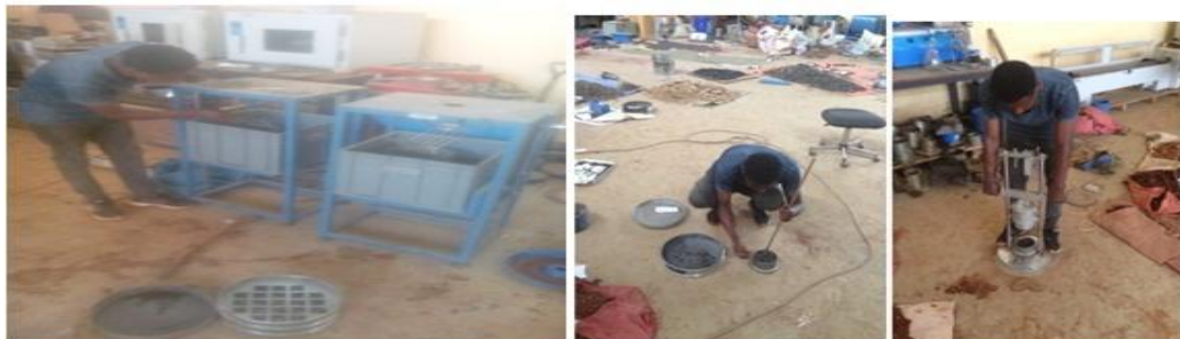
Figure 3.3 Specific Gravity test for RAP Aggregate and CA and Aggregate impact value test
