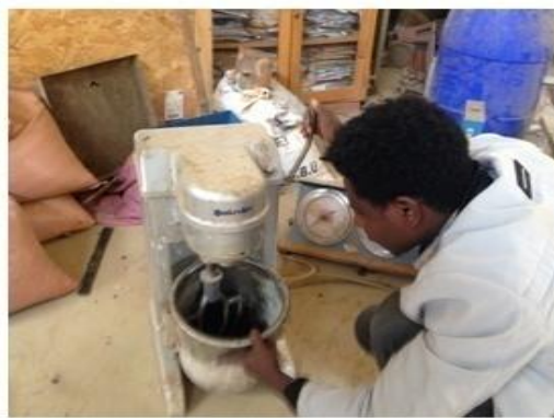
Figure 3.9 preparation of mold & heated and mixing by mechanical mixer
