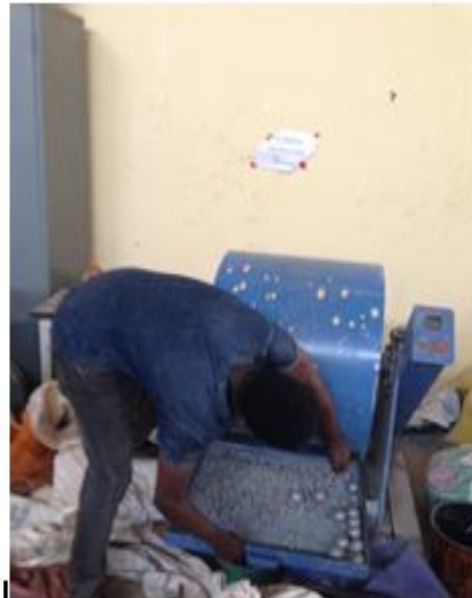
Figure 3.2 Aggregate crushing value and Los Angeles Abrasion test
