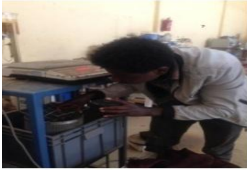
Figure 3.12 measuring of weight in Water and overnight cool of specimen respectively
