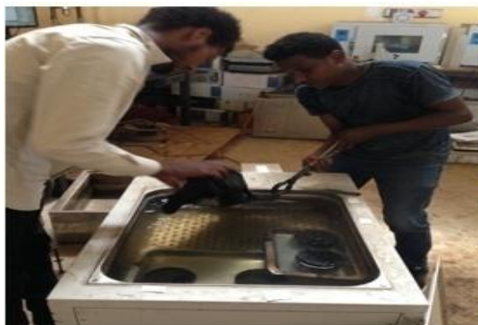
Figure 3.13 Prepare specimens for Test and Digital Marshall Flow stability test respectively
