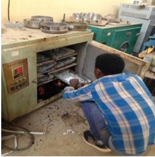
Figure 3.8 Drying of Aggregate and checking mixing temperature respectively
