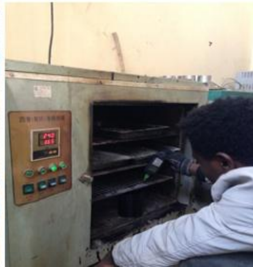
Figure 3.8 Drying of Aggregate and checking mixing temperature respectively
