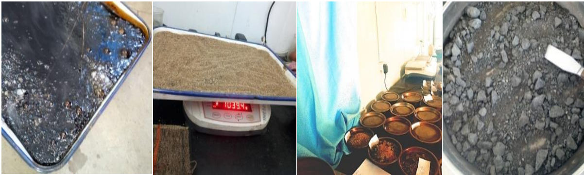
Figure 3. 5 Melting, Pulverizing, Adding and Mixing of Plastic Respectively
