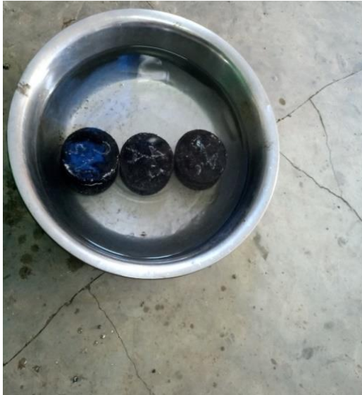
Specimens in water bath at 60 o c for 30 min
