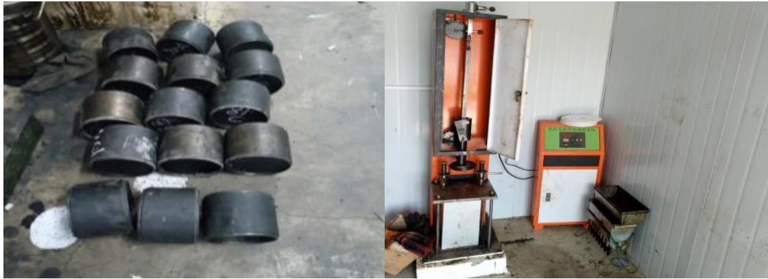
Figure 3.7 compacted modified specimen and automatic Marshall compaction machine
