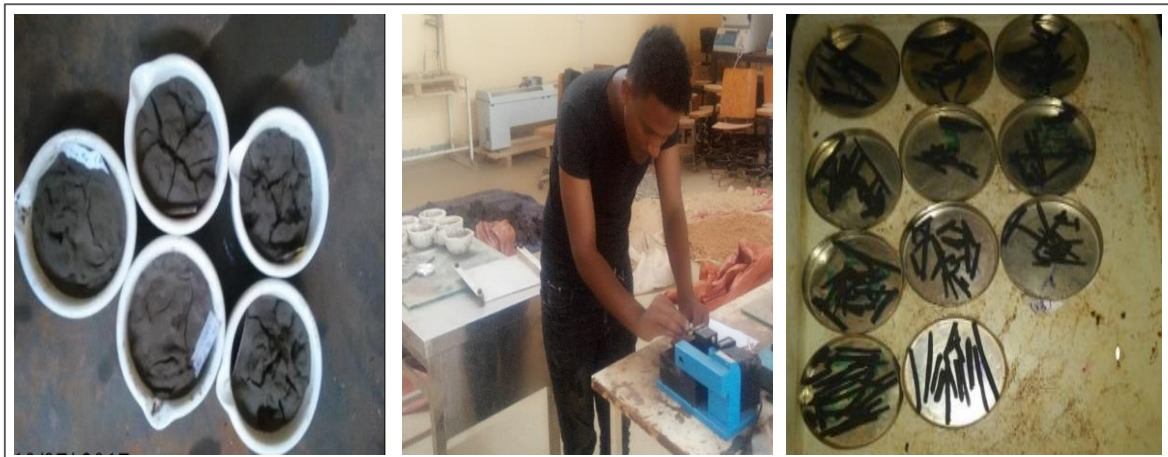
Figure 3.5: Atterberg limit determination (Source: Tariku A., 02/08/2018)
