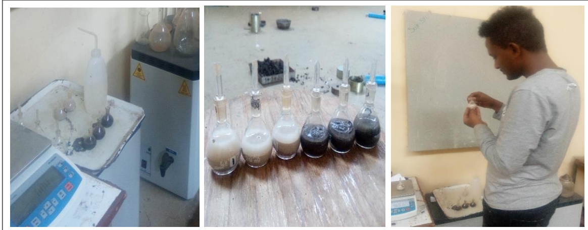
Figure 3.8: Specific gravity Test (Source: Tariku A., 28/07/2018)
