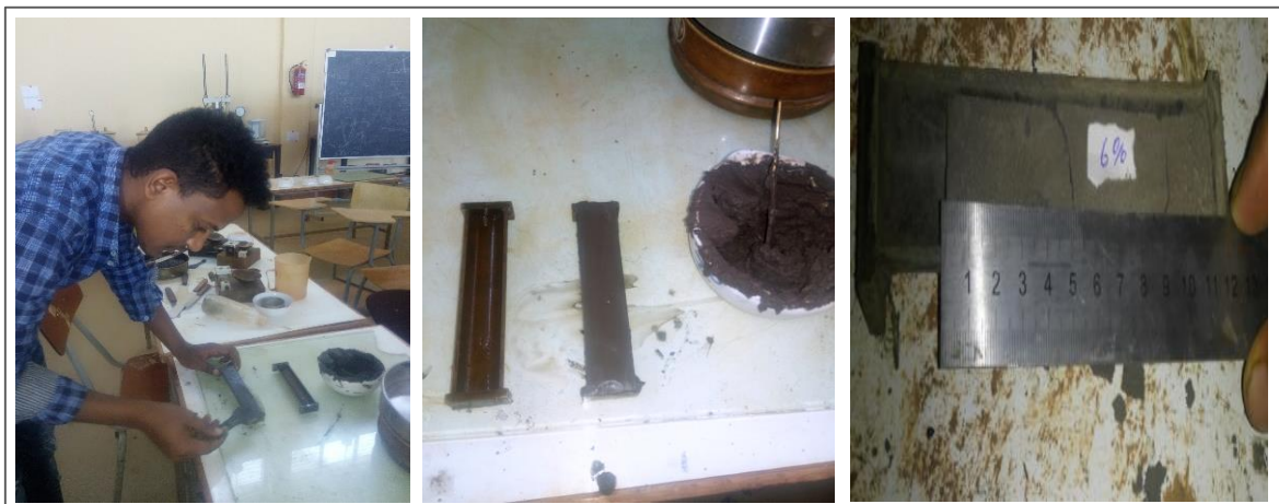
Figure 3.7: Linear Shrinkage Test (Source: Haile T., 05/08/2018)
