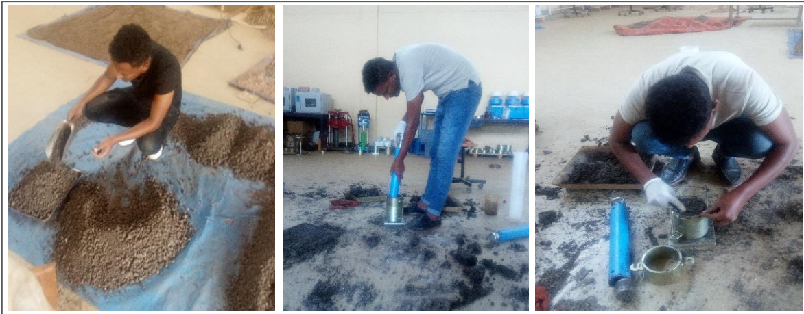
Figure 3.9: Compaction test and procedures (Source: Molla A., 16/08/2018)
