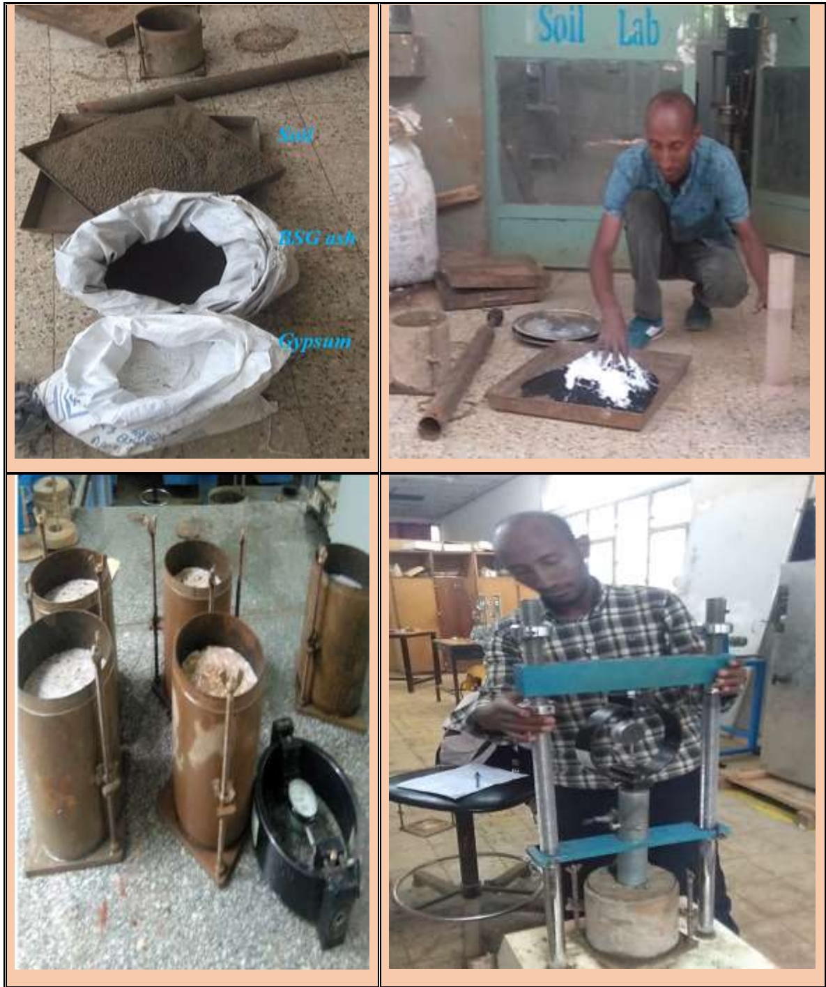
Figure 3. 7 Photographs for CBR test
