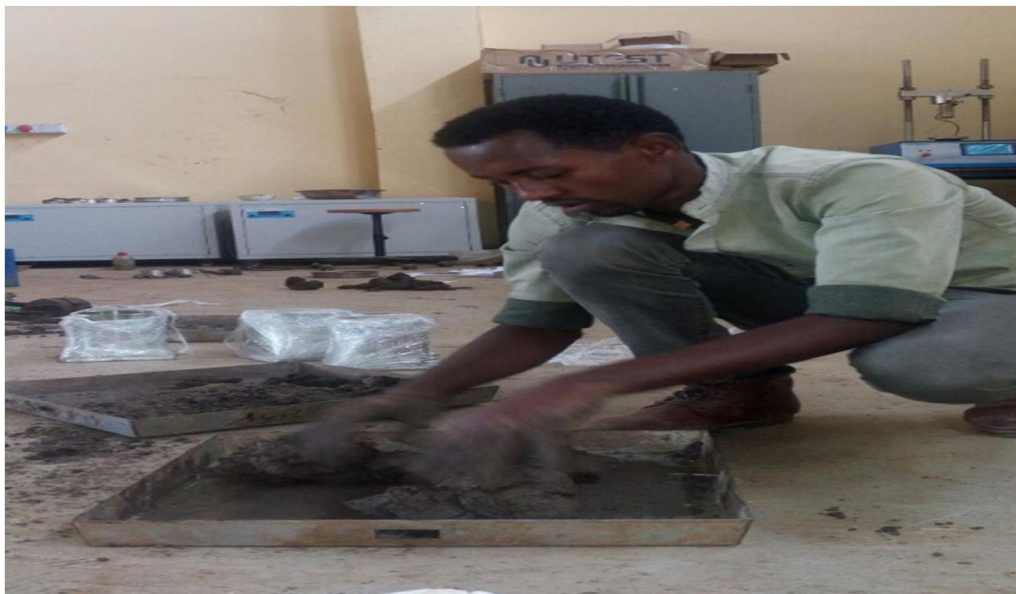
Fig 3. 4 Mixing of fiber and soil sample for CBR test (sep17,2018)
