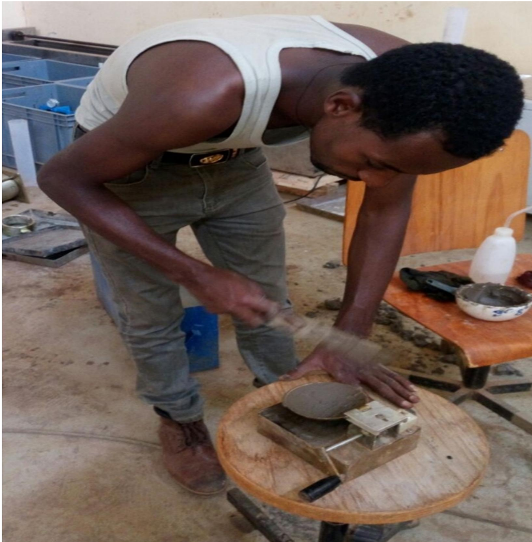
Fig 3. 6 Grooving of samples for LL test(sep 25,2018)
