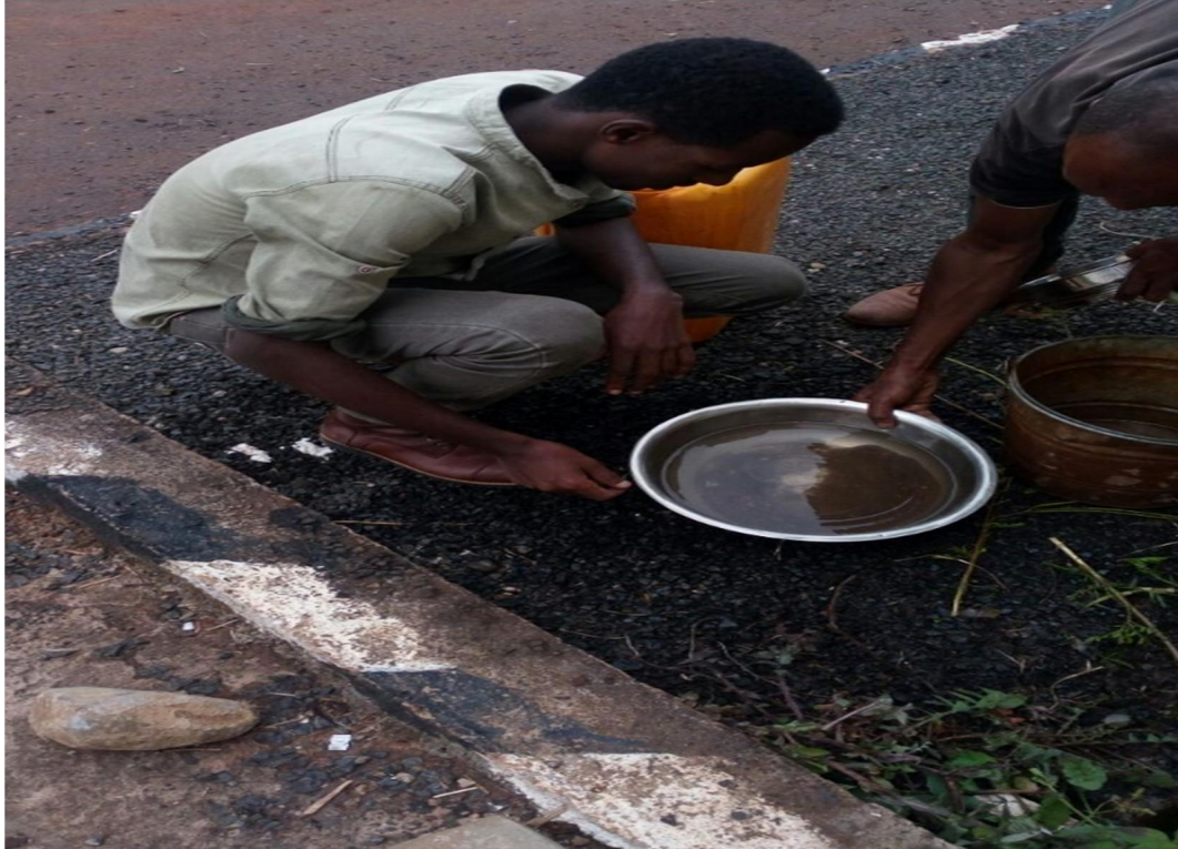
Fig 3. 5Washing of soil sample for wet sieve analysis test(sep 18,2018)
