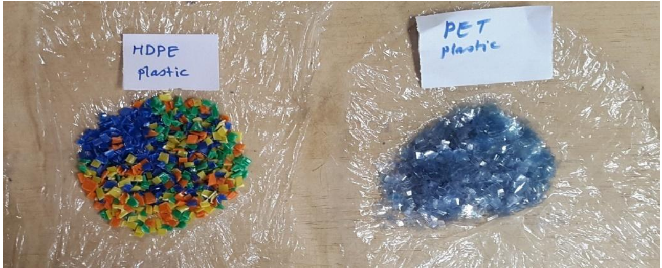
Figure 4- 2 Used Shredded Plastic Waste
