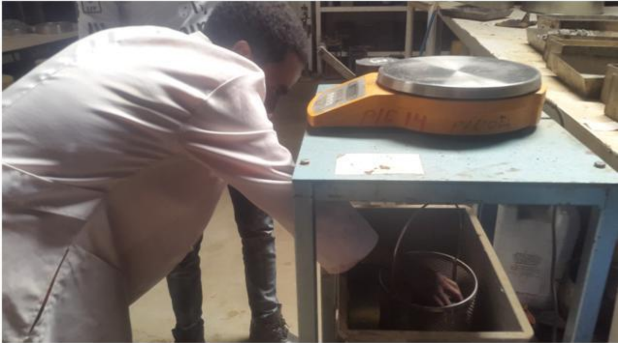
Marshal Samples weighting in water ( 19/05/2017)
