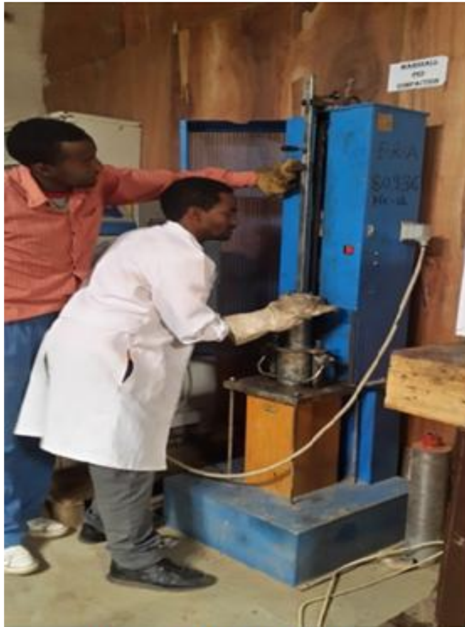
Compacting the mix by the Marshall Hammer (18/05/2017)
