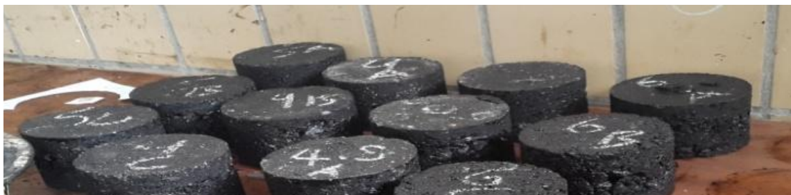
Figure 4- 3 Marshal Specimens with different bitumen content
