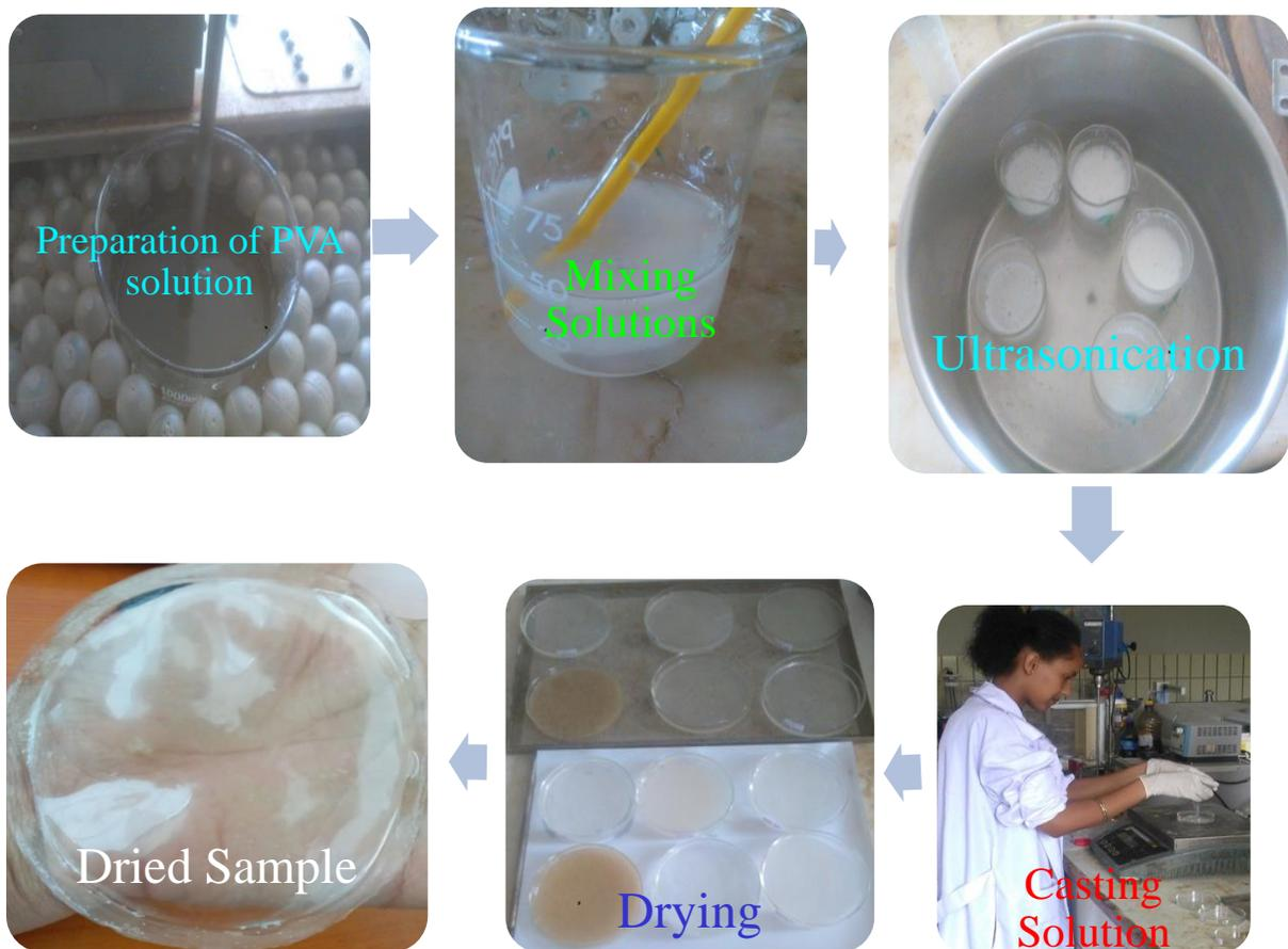
**Figure B-3:** Production process of PVA composite
