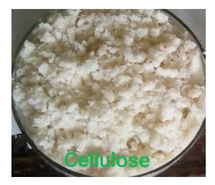
Figure 4.1: Produced cellulose after delignification and alkali treatment.
