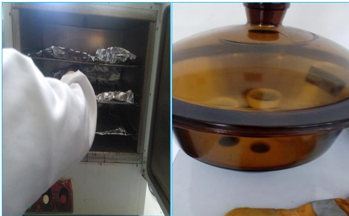
B.2 Prepared waste potato in oven and desiccators for moisture and ash content test
