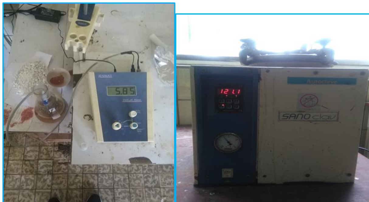
B.3 Mixture preparation and hydrolysis in autoclave
