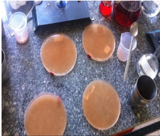
c Casting the gelatinized starch on petridish
