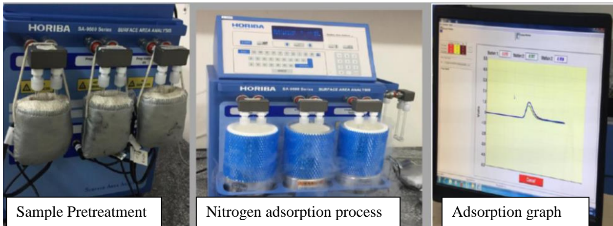
Figure B-6: Photo taken during sample treatment for BET surface area analysis
