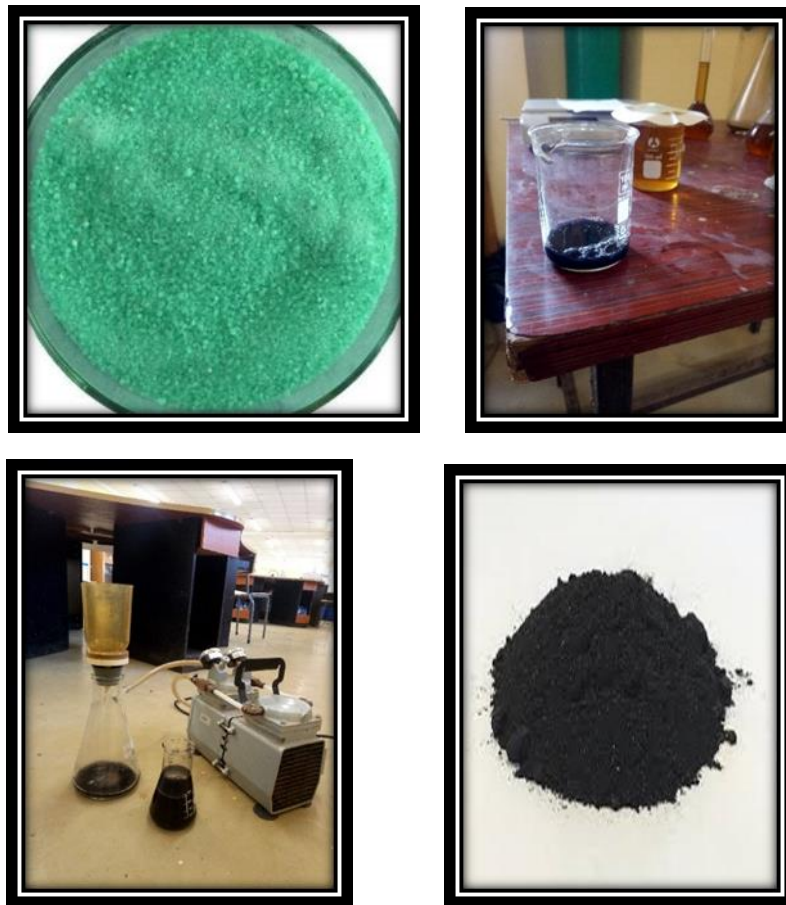
Figure A-3 Synthesize of nZVI using polyphenol extract
