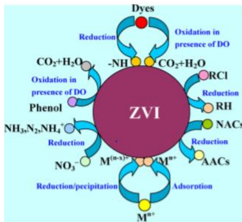
Figure 1 Schematic model of reaction mechanism of ZVI with different contaminants
