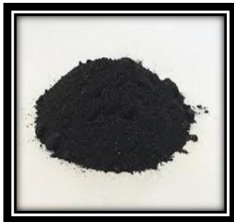
Figure 10 Synthesized nZVI using polyphenol
