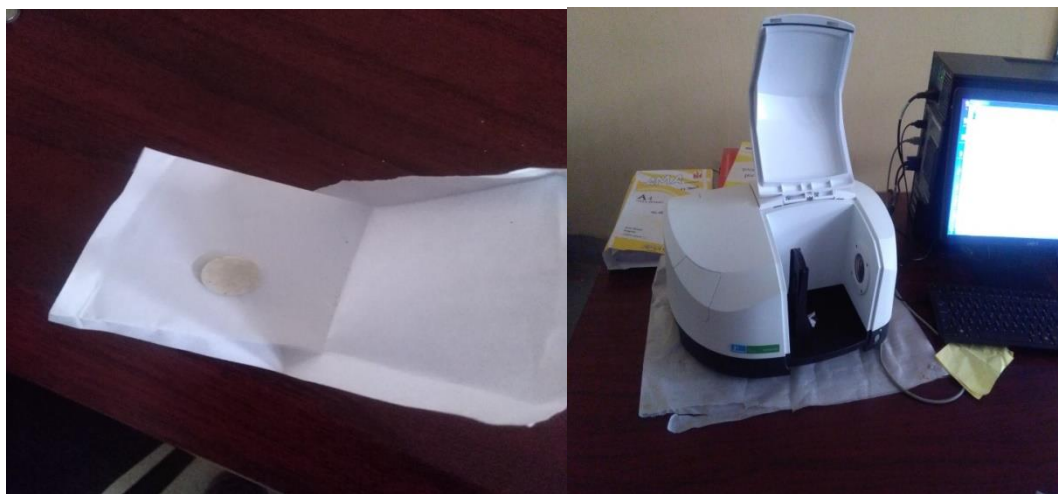
Figure 3.7 Pellet and FTIR analyzing machine
