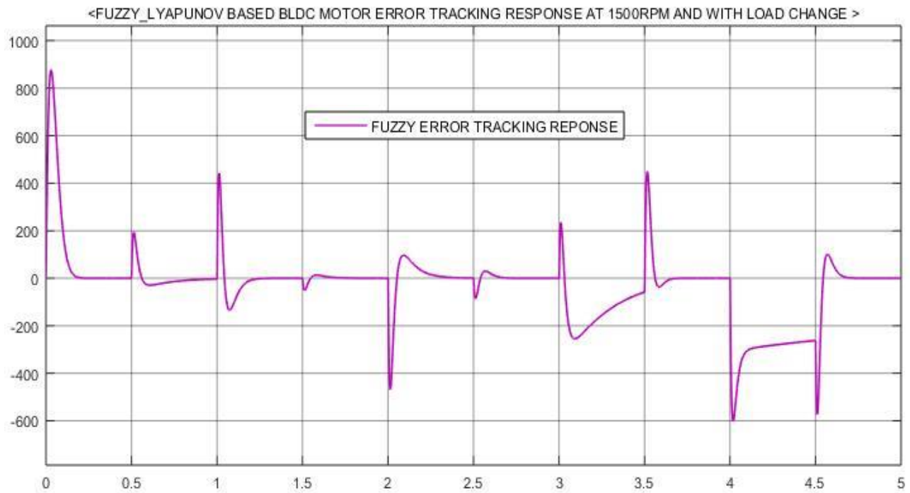
Figure 0.33 Error tracking response of Fuzzy based MRAC system with load change at rated speed
